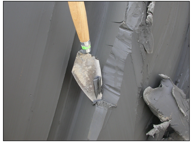
Figure 9. Massive grey clay seen in active borrow pits along Elleh Road near the confluence of the Fontas and Fort Nelson Rivers. The clay contains rare pebbles, in particular, granites of Canadian Shield provenance are present. Trowel blade is 20 cm long.
