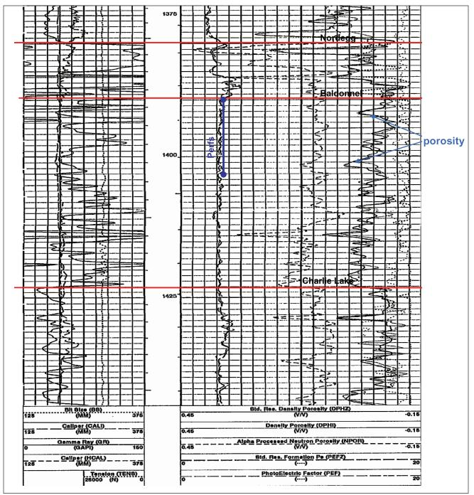
Figure 4: Neutron-Density Log d-25-G/94-G-1. Porosity is scaled in sandstone units, so through the perforation interval porosity peaks at roughly 8% when converted to limestone. Much of the interval is tight. The Pardonet Formation is missing, so the Nordegg Formation shale is acting as the seal.
