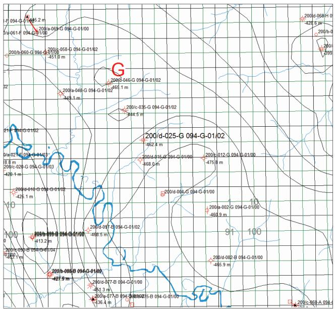
Figure 3: Structural Elevation of the Baldonnel Formation. Contour interval is 10 m. Structural elevations are shown below the well locations. Location d-25-G is shown to be in an intermediate structural position: it is between the elevation of the gas producers to the northwest (e.g., c-35-G) and the wet wells to the southeast (e.g., c-12-G). Although the scale of this illustration is not regional, it is possible to note the linear northwest-southeast trend of drilling and production.
