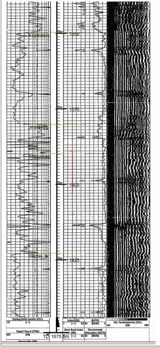
Figure 6: Cement Bond Log d-25-G/94-G-1. Generally strong amplitudes indicate good cement bond and low likelihood of leaks behind casing. Some weakness of bond is suggested by weaker returns at around 1380 m in the Nordegg Formation. Overlying bonds appear to be good, so leaks would likely not go far up-hole.
