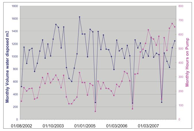
Figure 5: Water Disposal Plot for d-25-G/94-G-1. As volumes seem to be decreasing slightly, monthly hours on pump appear to be increasing. Data has been taken from the IRIS database of the Oil and Gas Commission of British Columbia.
