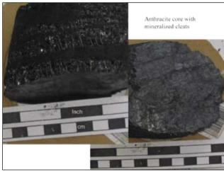
Photo 1: Anthracite sample prior to crushing, showing cemented face cleats and butt cleats.
