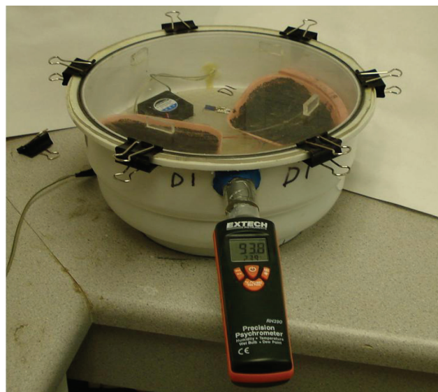
Figure 10: A desiccator with a relative humidity meter inserted. The desiccator contains two samples above a dish containing a salt solution that maintains a specific humidity.
