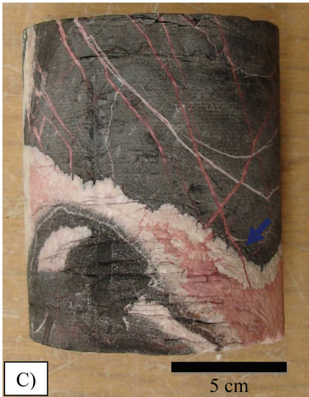
Figure 4. Core photos from D-16-A/94-N-15. A) Stained core photo showing the cross-cutting relationship between coarsely crystalline saddle dolomite, coarsely crystalline blocky calcite, dolomite-filled fracture, and calcite-filled fracture. 3798.0 m. B) Dolomite-filled fracture. 3810.9 m. C) Dolomite- and calcite-filled fractures as shown by Alizarin Red S staining. Notice calcite-filled fractures cut into saddle dolomite at the lower right corner (arrow). 3815.0 m. D) Open to partially open fracture post-dating coarsely crystalline saddle dolomite and blocky calcite. 3783.7 m.
