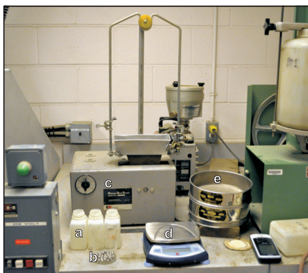
Figure 4. Equipment used in the experiments consisted of a) 250 ml plastic bottles; b) 10 mm, 3.6 g stainless steel balls; c) table shaker; d) scale; e) sieves.
