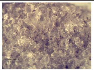
Close-up view at 20X magnification of a single chip. Fair to good textural relief indicates good intergranular porosity. Only minor detrital material is present among the predominant quartz grains.
