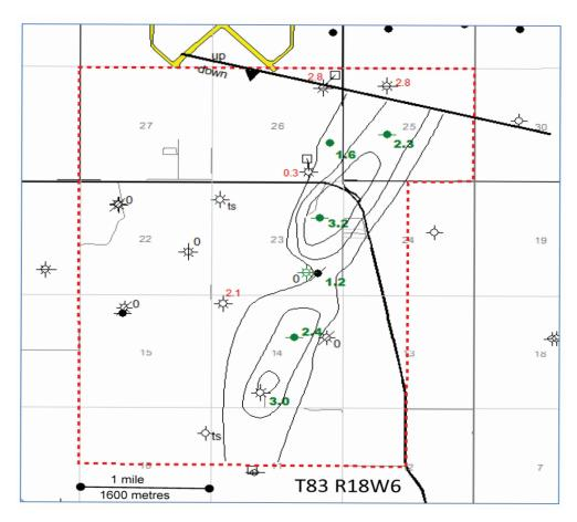
Figure 9. North Pine A pool; net oil pay North Pine member: Oil pay numbers are in green and gas pay is in red. Contour interval is 1 m net oil pay. The contours suggest a constriction in the central portion of the pool more or less coinciding with somewhat different pressure regimes between north and south. The extent to the south is not well defined. Faulting limits oil pay to the north.
