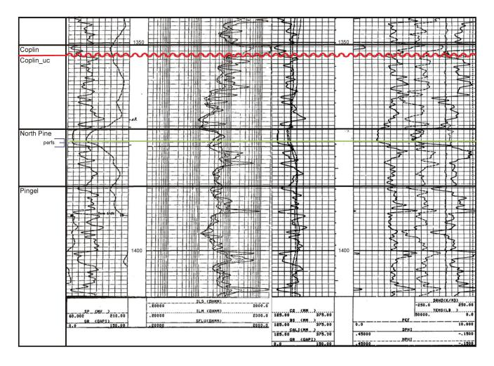
Figure 5. Location 8-26-83-18W6 induction and neutron-density logs: Neutron-density crossover in the North Pine indicates gas. This gas component has been important for the efficient 50% recovery rate of the pool. A gas-oil contact is at 1373 m measured depth (–706 m mean sea level).
