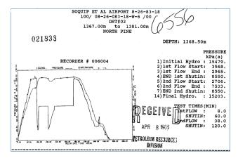
Figure 8. DST #2 at location 8-26-83-18W6. Very good to excellent permeability is displayed by almost immediate stabilization upon shut-ins. Oil (200 m) and water (100 m) were recovered.
