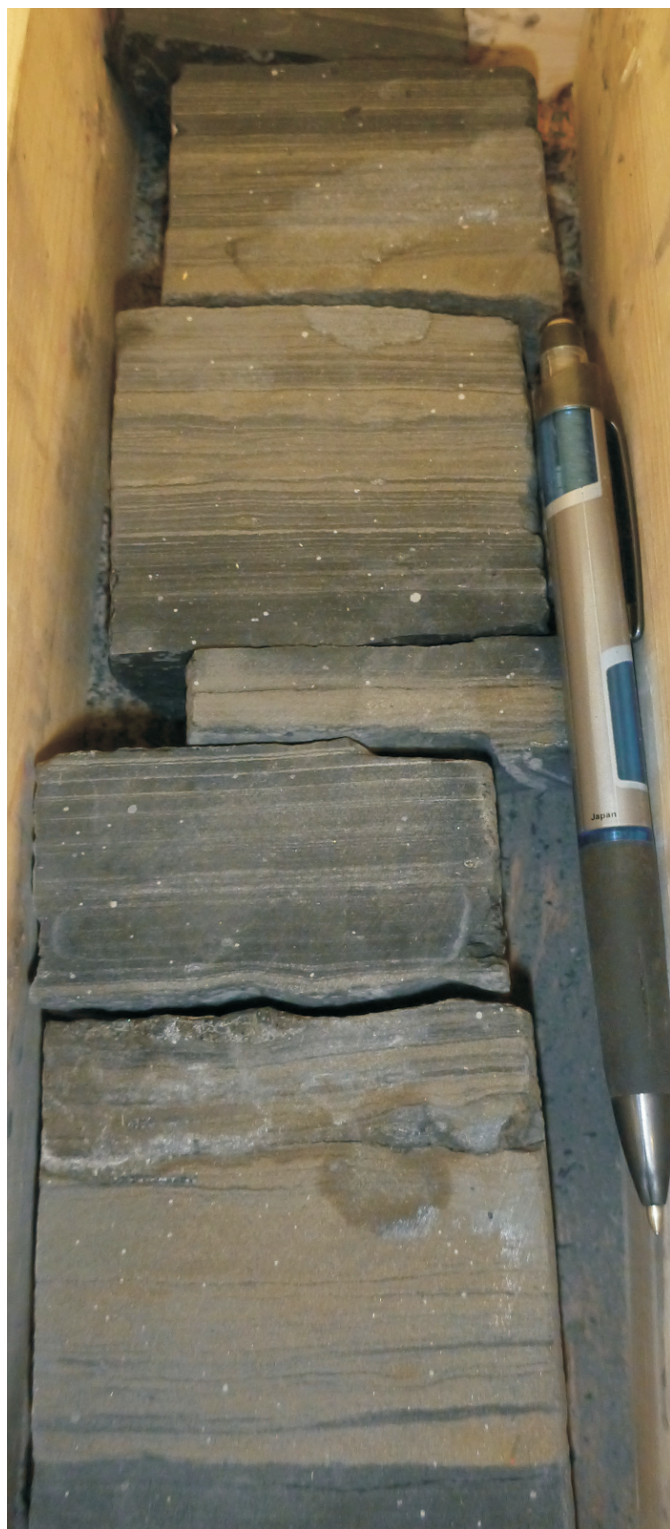
Figure 15: Fine- to medium- crystalline bedded pyrite (buff) horizon about 20 cm thick (top at 3777.17 m). Based on the correlation of the core gamma ray log with the downhole gamma ray profile, this horizon corresponds to the large gamma ray excursion at 3774 m on the gamma ray log, at the contact between the Patry member and the Fort Simpson marker (Figure 12). This pyrite likely formed in situ and, developed at the boundary where geochemical data suggest an oxic to anoxic switch, probably records changing redox conditions in the water column.
