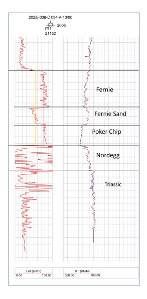
Figure 8. This Gamma Ray / Sonic log is a good example of Rock Creek (Fernie Sand) morphology, and one of the Rock Creek producers. Baseline gamma ray reading for Fernie shale is indicated by a red vertical line. The yellow line represents 30 API from baseline. Gamma Ray to the left of the yellow line was used to map Rock Creek clean sand. For location see Figure 4. BONAVISTA BLUEBERRY B-A036-C/094-A-13, Suspended Gas / Jurassic Rock Creek
