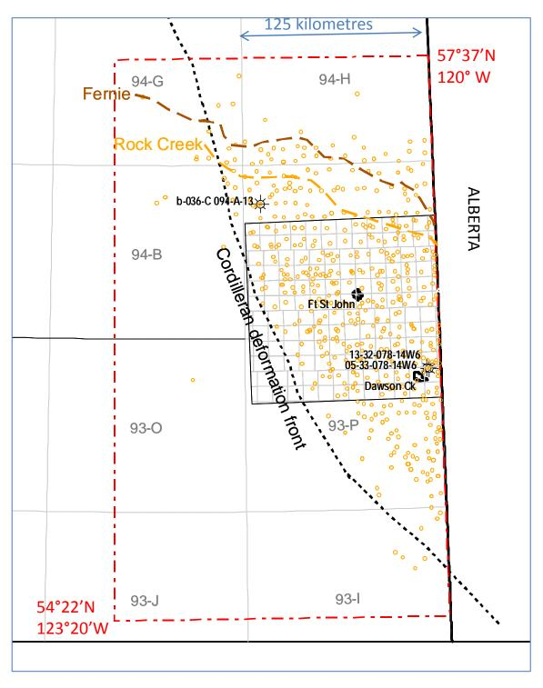
Figure 2. Three wells (b-36-C, 13-32 and 5-33) have produced gas or condensate from the Rock Creek Member (Fernie Sand) as designated by the British Columbia Oil and Gas Commission. Yellow dots symbolize wells with data used for this report. Fernie erosional edge is indicated; Rock Creek (Fernie Sand) can be either depositional or erosional.
