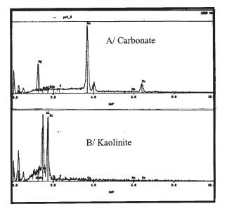
Figure 2. EDS scans of minerals in slits; A/carbonate and B/kaolinte.
