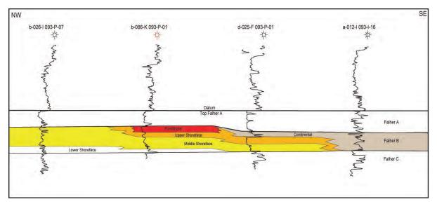
Figure 8. Cross-section illustrating progradation of the Falher B submember across the B.C. Deep Basin. Continental facies in the south pass northward to shoreface sandstones and conglomerates, which in turn grade to distal shoreface and offshore fine-grained clastics. Well b-86-K has produced >7 BCF from well-sorted foreshore and upper shoreface strata.
