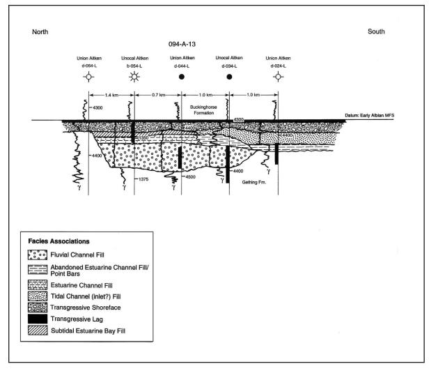
Figure 10. Cross-section across Bluesky estuarine valley fill at Aitken Creek. Fluvial channel conglomerates exhibit optimal reservoir quality; finer-grained estuarine to fluvial clastics are locally productive as well (from Alway and Moslow, 1997).
