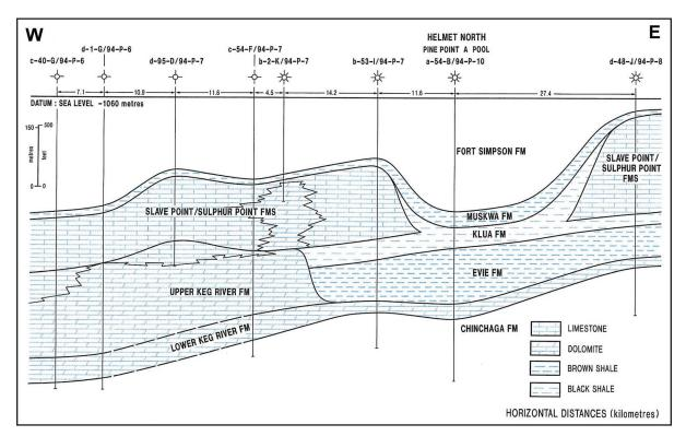
Figure 29. Schematic cross-section of Lower Keg River Platform Play in Helmet area, illustrating production from low-relief platform, basinward of high-relief Upper Keg River and Slave Point platform margins (from Reinson et. al., 1993).
