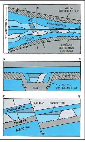
Figure 20. Normal faulting within the Fort St. John Graben complex played an important role in deposition of Kiskatinaw tidal/estuarine reservoir sandstones, and in formation of structural traps (from Barclay et. al., 1997).
