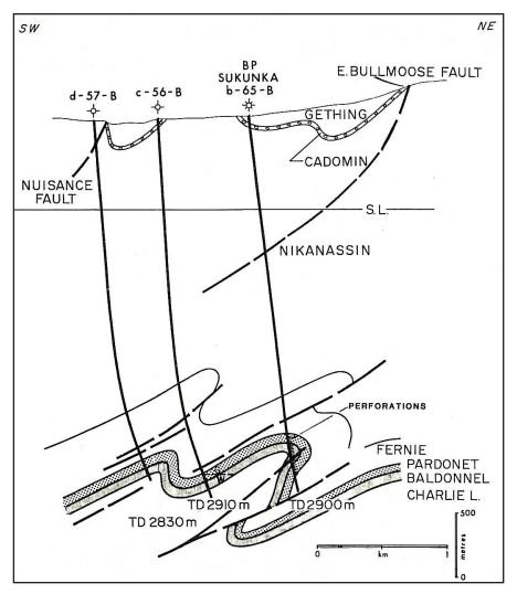
Figure 14. Baldonnel Fracture-dominant Foothills Structural Play at Sukunka, Southern Foothills Region (from Barss and Montandon, 1981). Tight Pardonet/Baldonnel strata are intensively fractured where extensional stresses are exerted over Foothills folds and faults. Wells penetrating fracture systems (as at b-65-B) feature high deliverabilities and reserves.
