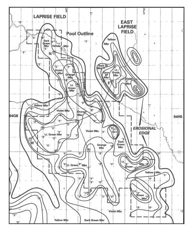
Figure 13. Situation map illustrating distribution of subcrop edges of members within Baldonnel Formation, Laprise and East Laprise areas (from Bever, 1990). Laprise and East Laprise are good examples of Baldonnel subcrop traps, preserved beneath the pre-Cretaceous unconformity, and sealed primarily by Cretaceous marine shales.
