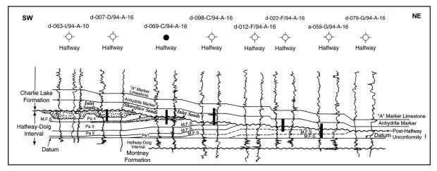
Figure 16. Stratigraphic cross-section at Peejay, illustrating discontinuous preservation of Halfway tidal channel and shoreface sandstone reservoirs (from Caplan and Moslow, 1997).
