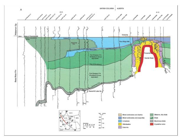
Figure 26. Schematic regional cross-section, illustrating Leduc reefal buildups flanking Peace River Arch in northwestern Alberta and adjacent B.C. (from Switzer et. al., 1994).
