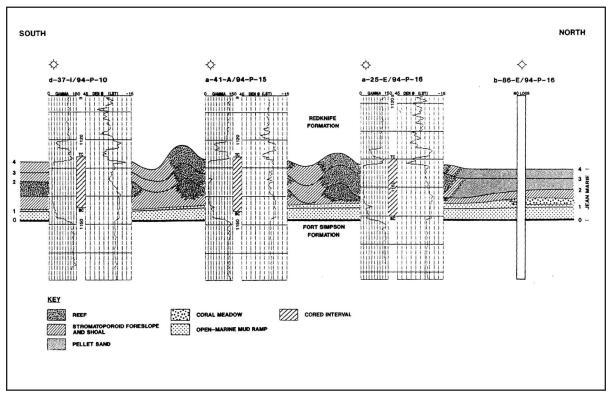
Figure 25. Stratigraphic cross-section, Jean Marie Formation, Helmet area (from Stoakes, 1992). Note patch reef stratigraphic sweet spots developed within different depositional cycles, encased in tighter foreslope and shoal facies.
