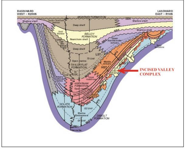
Figure 19. Schematic regional cross-section of Carboniferous – Permian strata across Fort St. John Graben area (from Barclay et. al., 2002). Belloy reservoirs are best developed in shallow marine sandstone and carbonate units deposited on the flanks of the graben complex. Taylor Flat strata consist of open marine carbonate and fine clastic strata, with relatively poor and discontinuous reservoir development. Fluvial to estuarine sandstones of the Kiskatinaw are locally important reservoirs.
