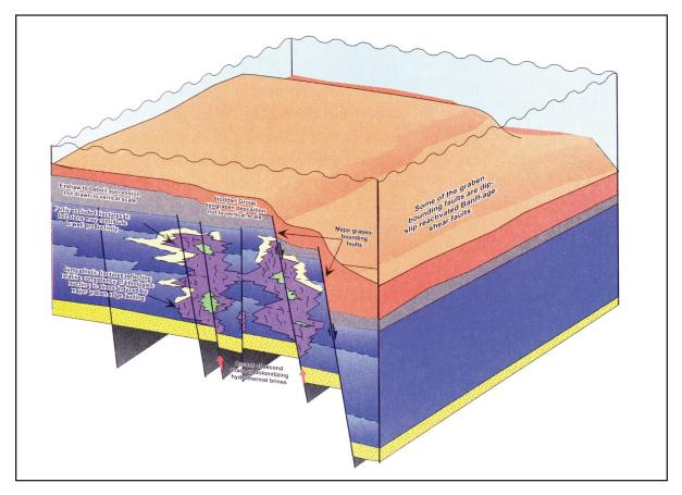
Figure 23. Schematic block diagram illustrating development of hydrothermal carbonate and chert reservoirs within the Wabamun Group, as the result of migration of hydrothermal brines along block faults (from Packard et. al., 2001).
