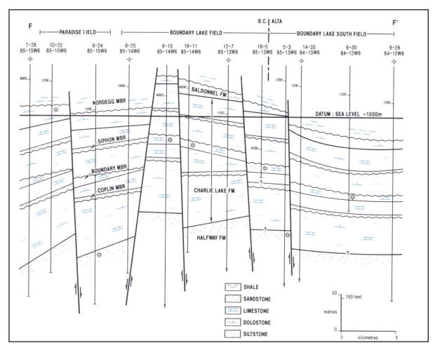
Figure 15. Structural cross-section through Charlie Lake Formation across the Fort St. John Graben area. Note development of reservoir sandstones and carbonates associated with regional unconformities within the Charlie Lake, and importance of faults as structural traps.
