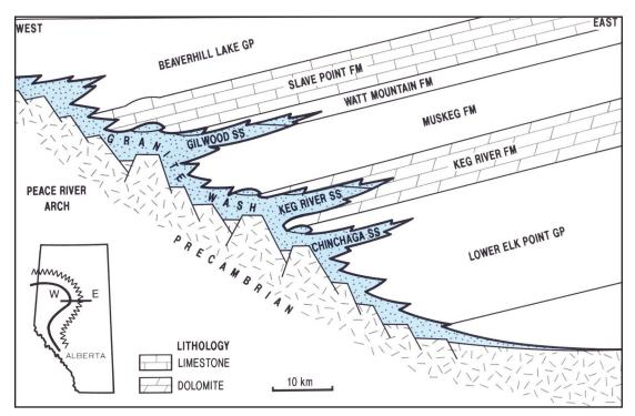
Figure 28. Schematic regional cross-section, illustrating Granite Wash sandstone reservoirs mantling Peace River Arch, with sandstone tongues corresponding to specific regressive pulses correlated basinward (from Reinson et. al., 1993). Reservoir distributions have been mapped in Alberta, but are more speculative in B.C.
