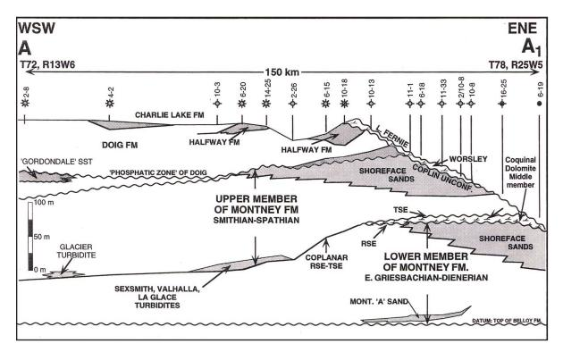
Figure 18. Schematic regional cross-section, Montney Formation (from Moslow and Davies, 1997). Shoreface sandstone reservoirs to the east produce in the Subcrop Edge – Proximal Sandstone Play in the Fort St. John and Fort Nelson Regions. Further basinward, distal shoreface (not specified) and turbidite sandstone plays are current exploration targets in B.C.
