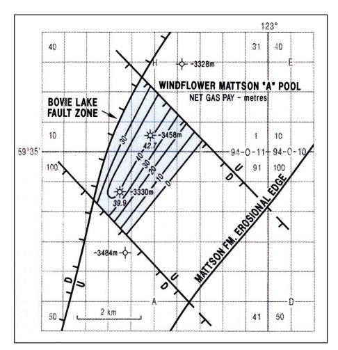
Figure 21. Structural trap in Mattson sandstones along the Bovie Lake Fault Zone, eastern margin of Liard Basin (from Barclay et. al., 1997).
