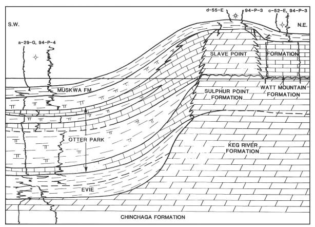
Figure 27. Cross-section illustrating platform margin reef reservoirs in the Slave Point Barrier Reef / Pinnacle Play of the Fort Nelson Region (from Lehto, 1990).
