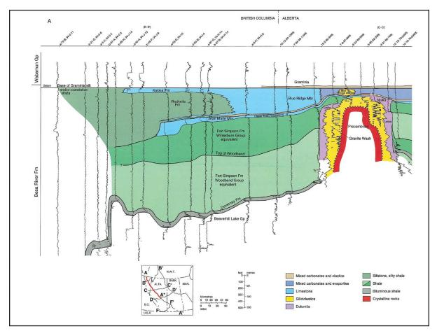
Figure 24. Schematic regional cross-section, illustrating development of Kakisa platform carbonate reservoirs in northeastern British Columbia (from Switzer et. al., 1994).
