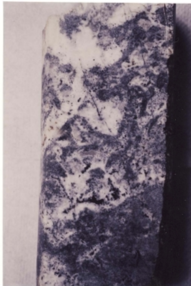
b. c-94-L/94-J-7 6476.5 ft. Upper Slave Point Pseudobreccia with three phases of dolomite. Fabric preserving skeletal peloid grainstone with some areas light grey pyrobitumen speckled destructive replacement dolomite with areas of dissolution infilled by white cement. Note fragmentary pyrobitumen caught up in cement.
