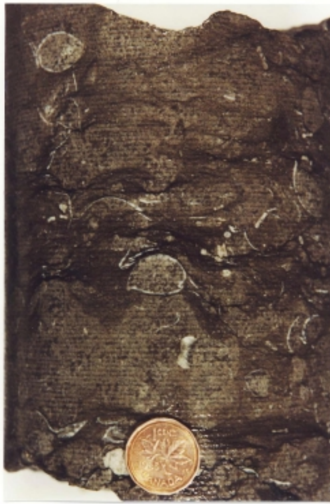
b. 11-4-97-5W4M 2283.3m Slave Point Skeletal wackestone with nodular boudinage structure and sparse crinoids and brachiopods.
