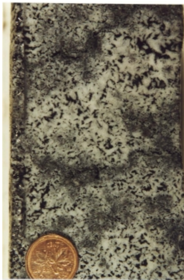
b. a-99-K/94-P-4 6926.3 ft. Slave Point Grey fabric destructive dolomite with characteristic dark interstitial bitumen. Note the gradation in grain size away from stylolite surface where replacement was initiated. Also total destruction of earlier fabric of limestone other than vestigial and disrupted solution planes.
