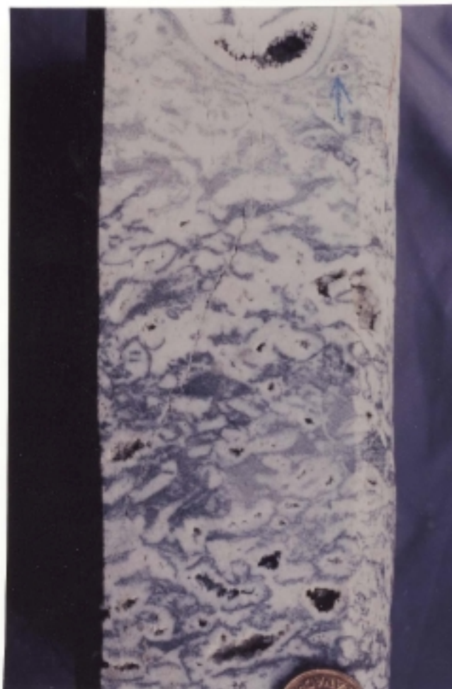
b. a-61-F/94-J-10 6706.0 ft. Middle Slave Point Dolomite with relict grey fabric preserving dolomite and extensive intrafossil cementation by white saddle dolomite. Dendroid stromatoporoid boundstone.
