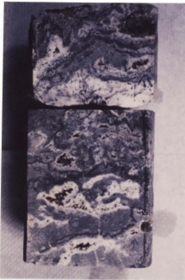
a. c-94-L/94-J-9 6491.0 ft. Slave Point Dolomite, three generations. Early fabric preserving with intrafossil voids. Bladed destructive replacement of fossils, and white cement in intrafossil vugs. Bulbous to dendroid and laminar stromatoporoid floatstone.
