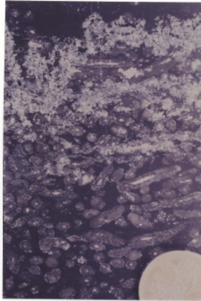
b. c-56-L/94-J-9 6425.5 ft. Slave Point Amphipora , Thamnopora floatstone with dense bed of Amphipora rudstone with replacive fabric destructive saddle dolomite.
