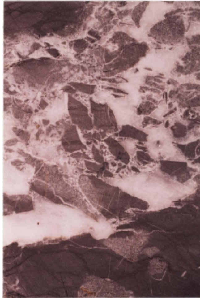
b. a-67-D/94-O-13 17,113.0 ft. Chinchaga Dolomite microcrystalline breccia. Dark bioturbated mudstone disrupted angular fragments, some internal sediment of fine angular chips, rimmed by fine layer saddle dolomite, infilled by calcite.
