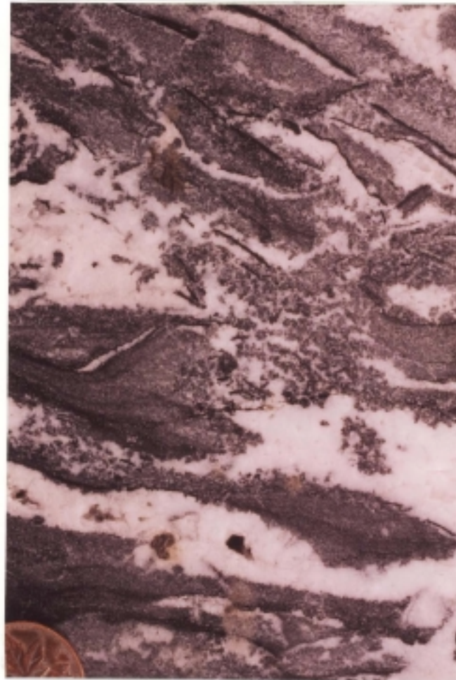
b. a-67-D/94-O-13 17,140.0 ft. Chinchaga Algal laminate and peloid grainstone. Disrupted fabric caused by displacive, replacive anhydrite cement now white saddle dolomite.
