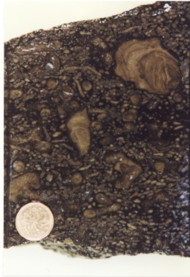
b. c-3-C/94-J-11 6420.5 ft. Slave Point Dendroid and bulbous stromatoporoid with coated grains and Amphipora rudstone in bituminous mudstone.
