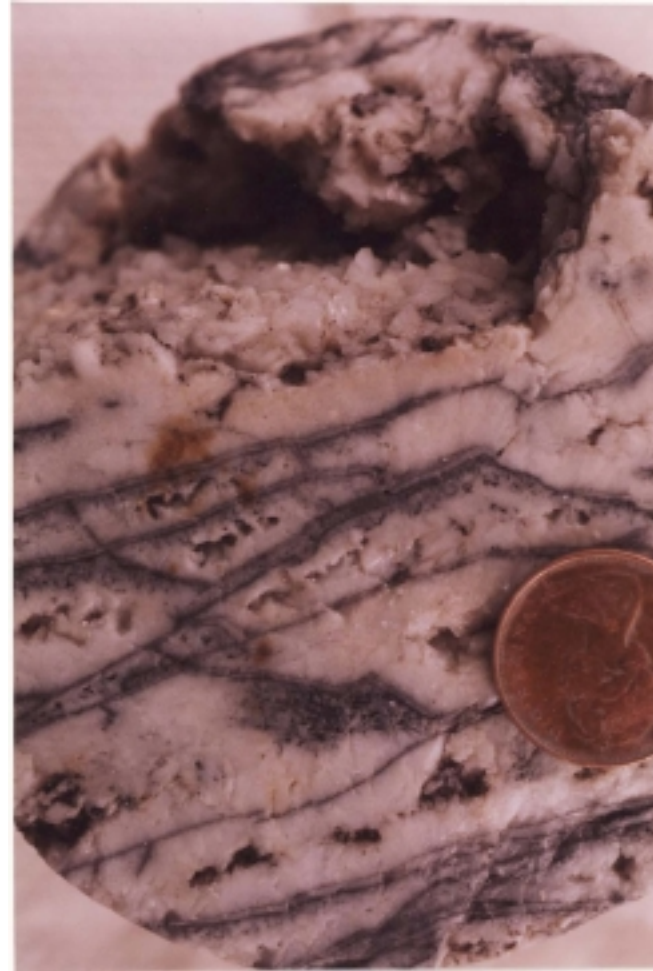
b. c-14-G/94-J-13 9987.5 ft. Chinchaga The same example as Plate 59(c) viewed by upper surface. Note vertical distribution of vugs in white dolomite.
