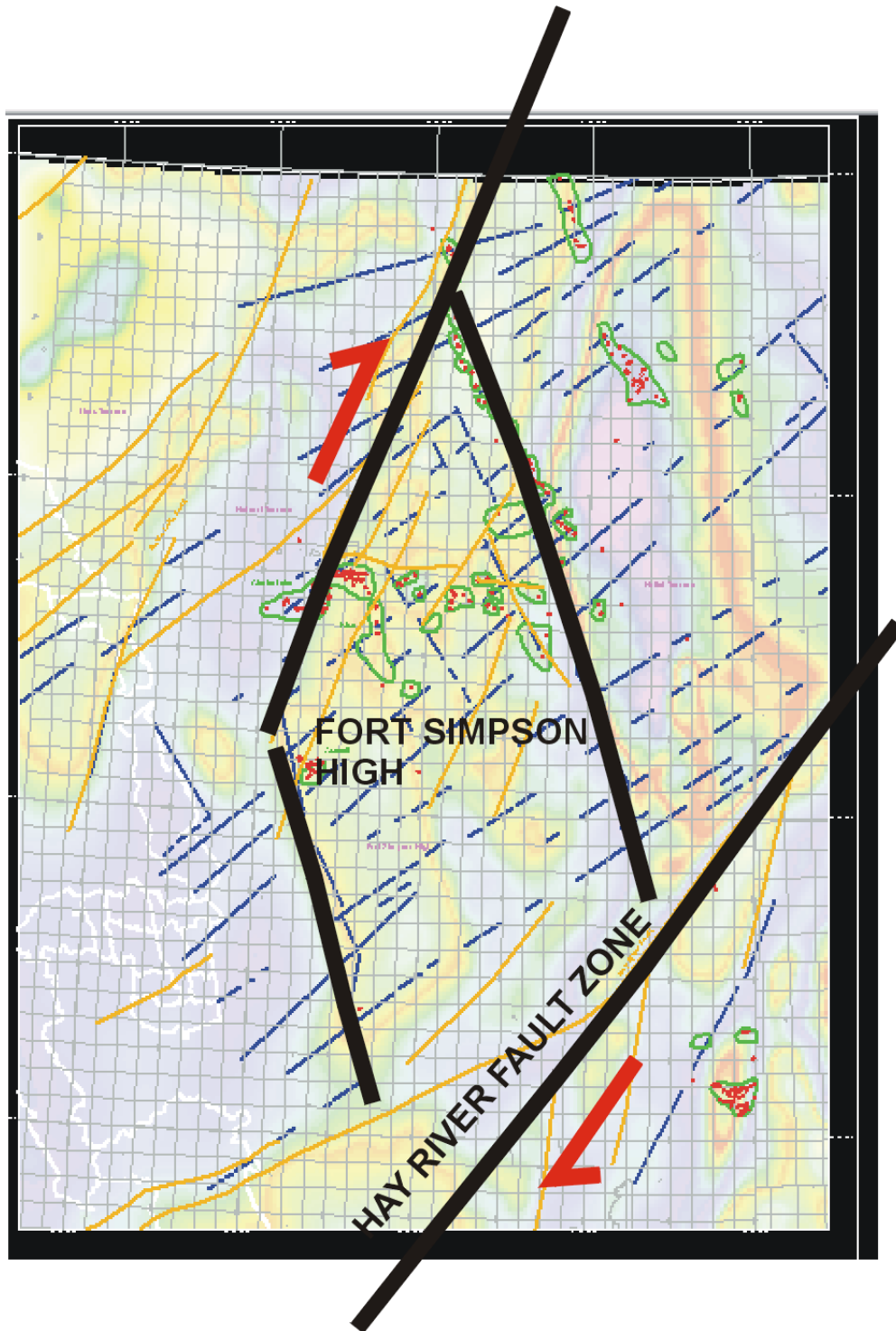
Figure 3. Interpretation of Fort Simpson High as “push-up” structure in a left stepping right-lateral strike-slip fault zone.
