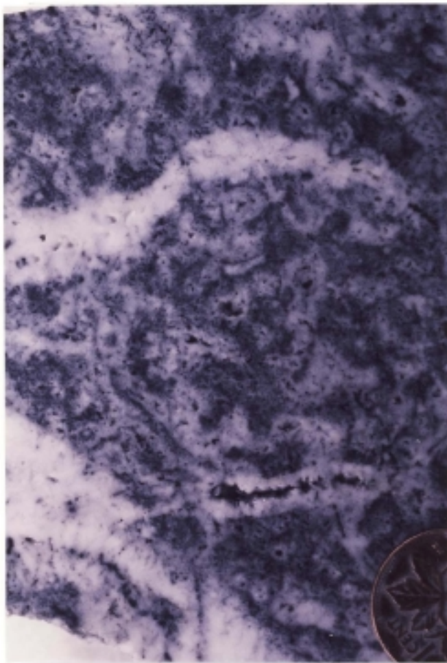
a. c-94-L/94-J-9 6434.5.0 ft. Upper Slave Point Three generations of dolomite: 1) Dark fine crystalline rhombic matrix, early burial type dolomite. 2) Light grey bladed metasomatic dolomite replacing some relict fossil coenostea. 3) White megacrystalline dolomite cement infilling void space created by dissolution of calcite.
