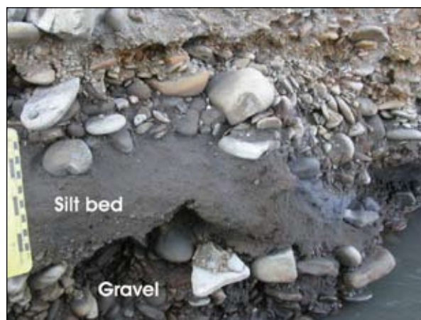
Figure 14: Deformed silt and fine sand bed within the lower gravel at site MT04-115.
