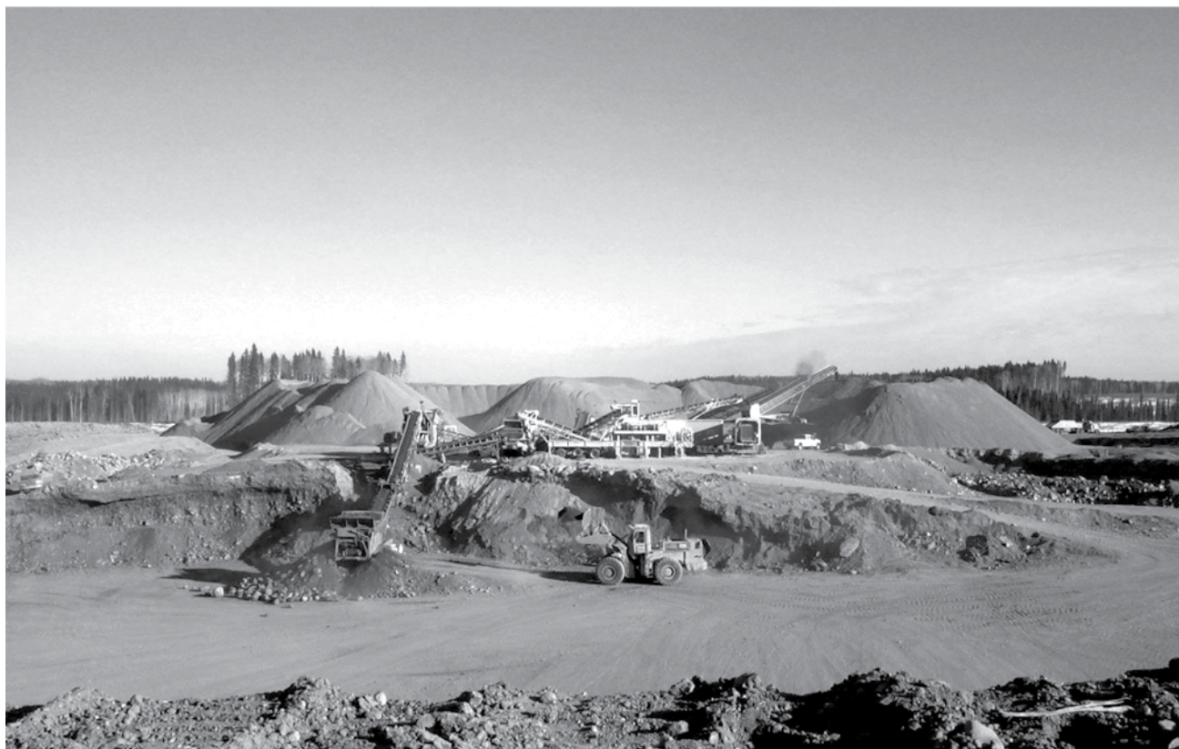
Figure 2. Active gravel mining operation during the winter of 2004 at the Elleh deposit. Aggregate from the operation was stockpiled at various locations for use on the SYD and Clarke Lake Bypass Roads. Gravels in the area are extensive and include mainly glaciofluvial gravels deposited during the last glaciation. (Photo provided by Quentin Huillery, Leducor CMI Ltd.)
