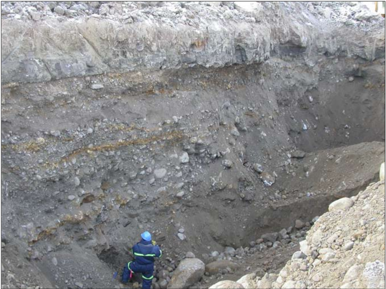
Figure 3. February 2005 exposure in the southwest corner of the Kotcho East gravel pit, operated by EnCana Corporation. Buried gravels in the area are up to several metres thick, and the overlying clay-rich sediments are typically 1 to 2 m but up to 5 m thick. The upper part of the overburden has been stripped here, and the base of the gravel is below the base of the exposure.
