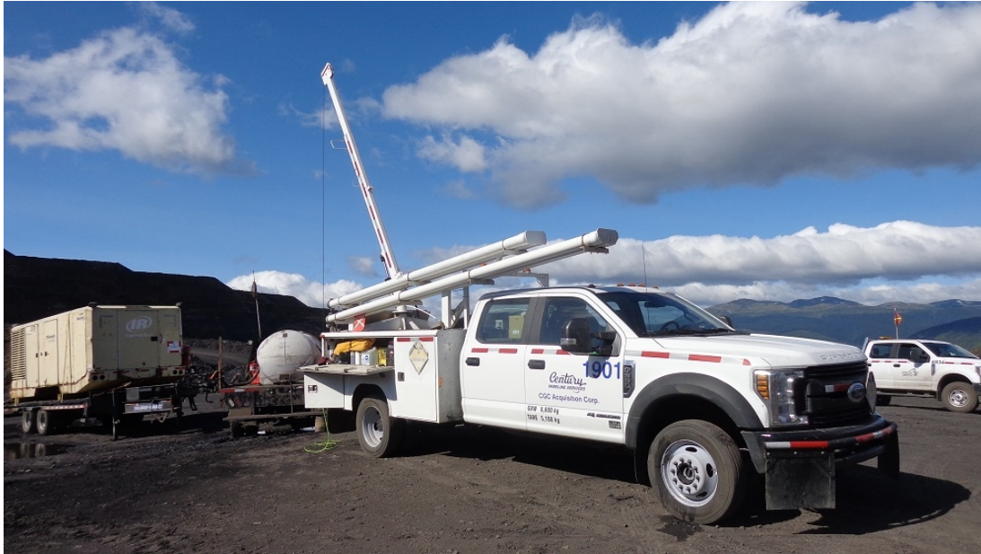
Plate 2: Century Wireline geophysical logging unit, with extended-reach sheave-boom and overhead storage tubes for wireline sondes. To left are trailer-mounted air-compressor and flat-deck truck with water tank. [RC5473a/20.jpg]
