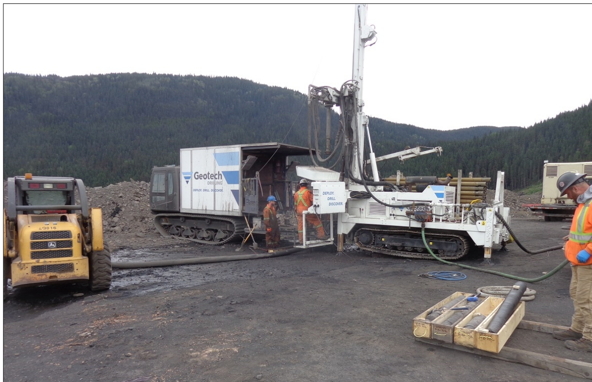
Plate 1: Fraste DR-3 drilling rig set-up for coring. From left to right: skid-steer loader, track-mounted supply/workshop van, track-mounted drill with integral rod rack and rod-handling manipulator, core in core-boxes (with one box containing overbored length of solid rock core), and trailer-mounted air-compressor. [RC 5485a/20.jpg]
