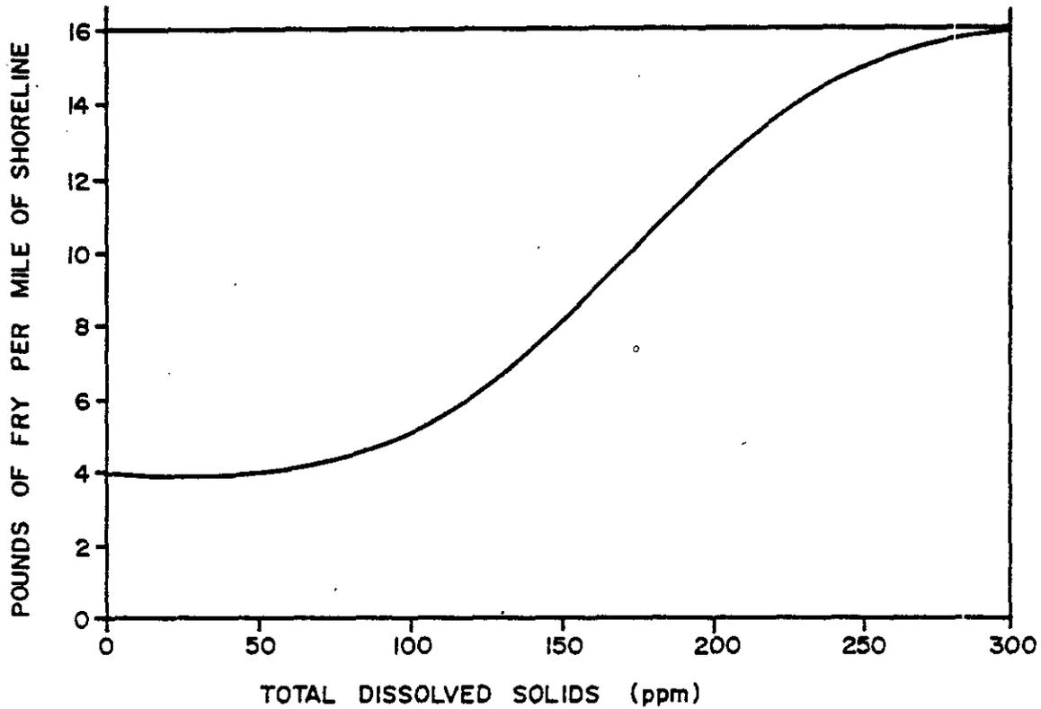
Curve used to estimate Rainbow Trout fry stocking rate from total dissolved solids (from Smith *et al.*, 1969)
