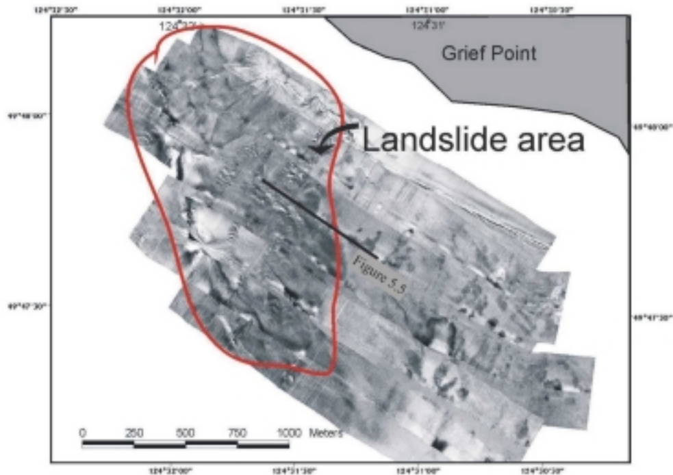
Figure 5.3 Sidescan sonar mosaic of the Grief Point landslide. Water depths range from 20 m in the north to 220 m in the southwest area of the image (from Mosher et al. 2001).
