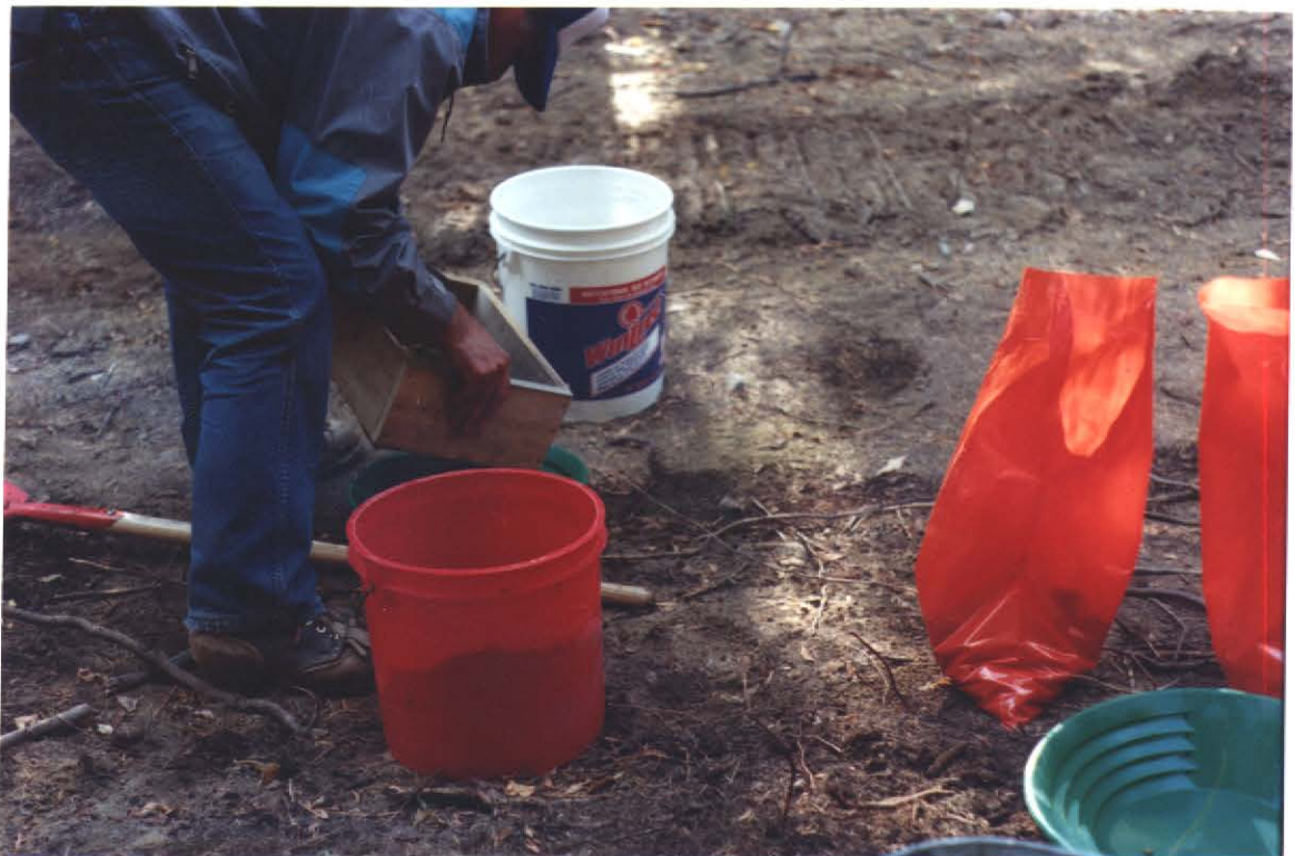
Photo 25- Samples were screened using a 1/4 inch minus classifier and either panned out on site/ and/or taken in plastic bags back to Grand Forks for panning.
