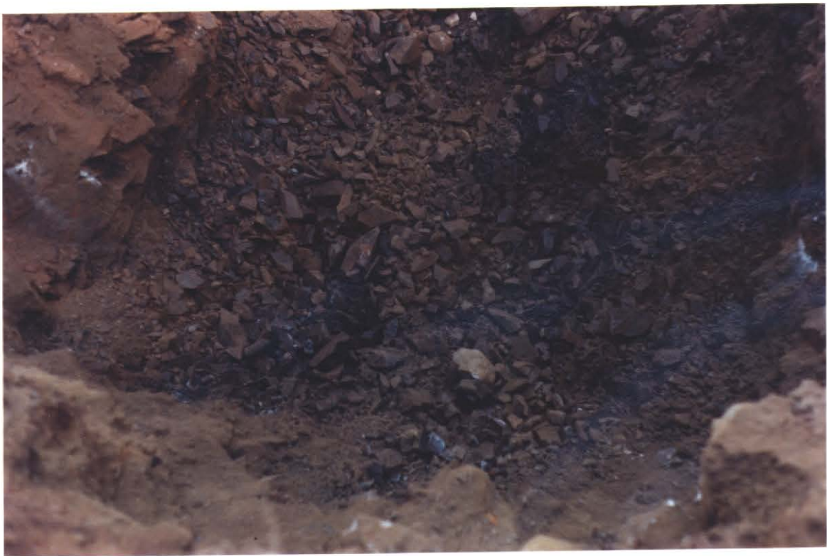
Photo 19 - Soft shale bedrock encountered on the Sites "D, E, and F"
