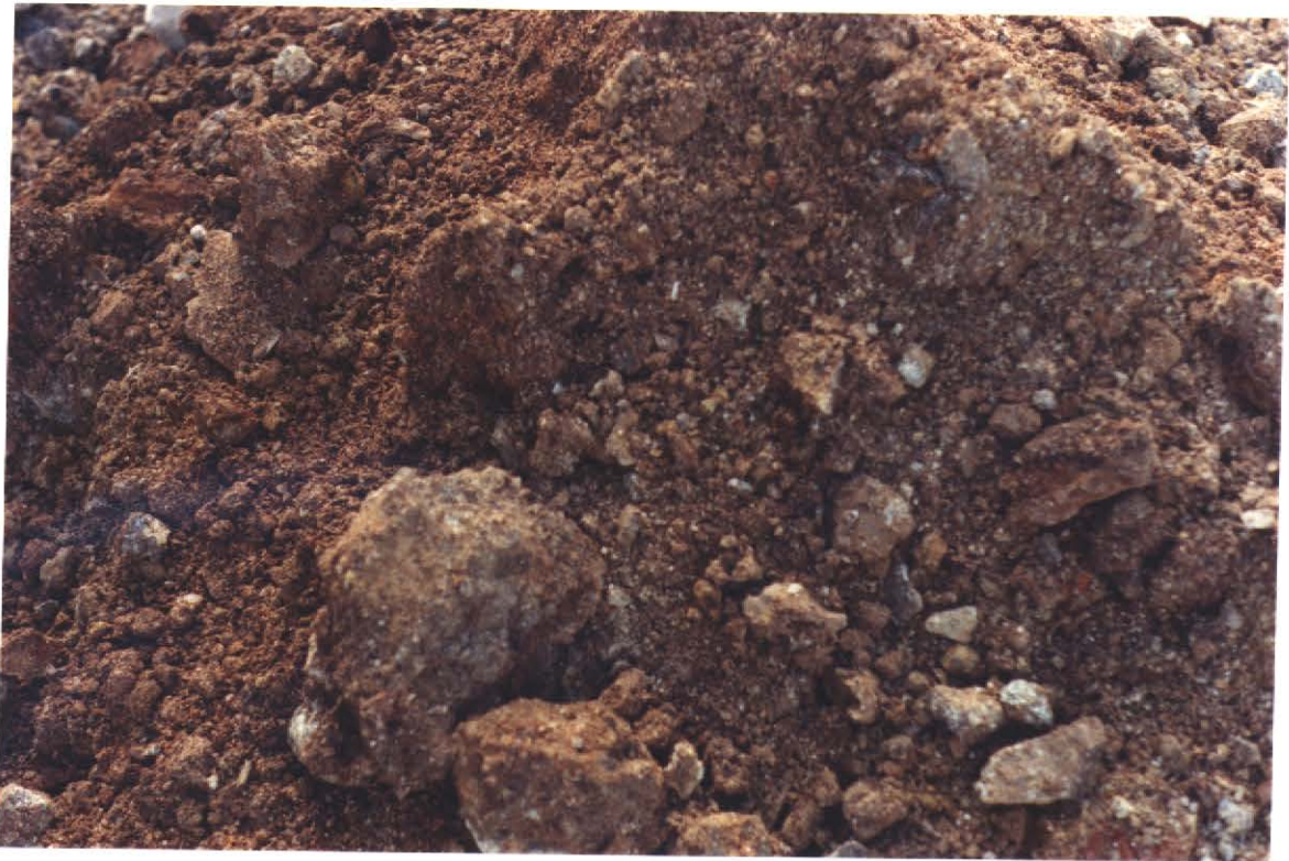
Photo 16- At Site "C" from about 3.5 meters to 7.0 meters depth a red sulphide type of granular material ( red goo ) The material contained no free gold, and unfortunately a sample was not sent away for metallic assay
