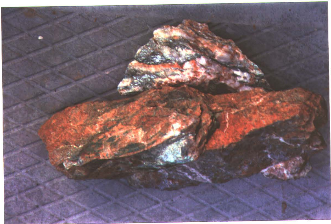
Photo 4b: Sample #5 -- fuchsite in carbonate breccia
