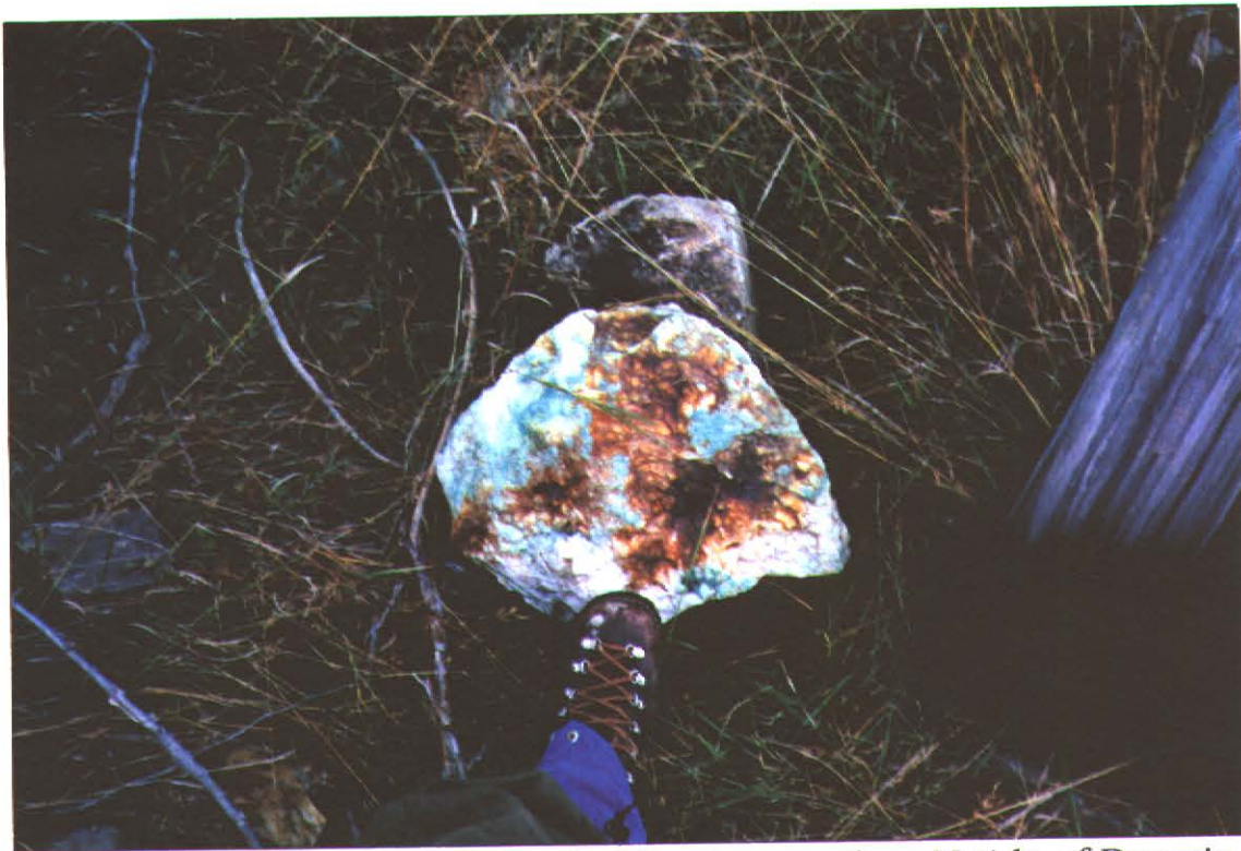
Photo #4- Located at east end of logging road on N side of Downie Ck. see map 3-2. Quartz float containing pyrite, chalcopyrite and malachite.
