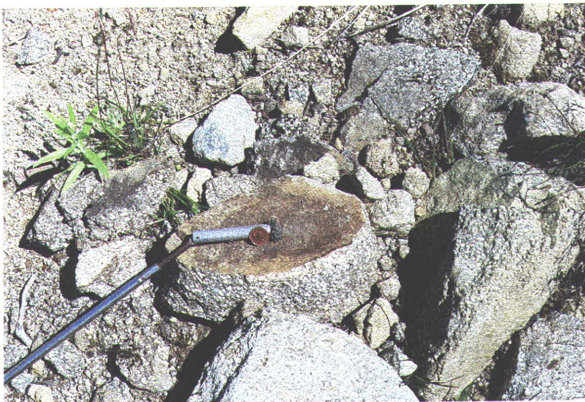
Fig. 3. Biotite-Hornblende-Quartz Diorite of the Ruby Range stock, on Magnetic Hill. Note the abundant magnetite collected from the soil on the end of the magnet (penny is for scale)
