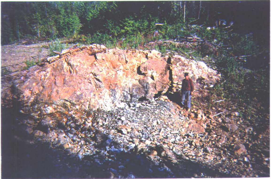
Cam/Gloria - Trench #1 - Photo #1 Quartz vein exposed along strike. Camille standing on rock pile. Picture view taken against strike
