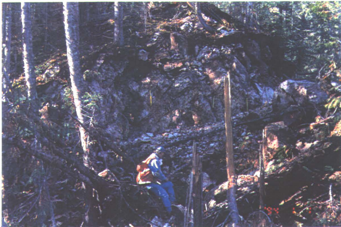
Trench # 2 Showing survey ribbons nailed to the quartz vein Tag # 95126 to 96132 (one metre intervals). Tag 95130 assayed Au 7.12 g/t, Tag 95129 assayed 2.65 g/t
