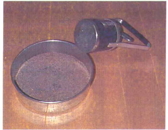
Photo3 – Hand magnet used to separate magnetite and pyrrhotite grains from the samples.
