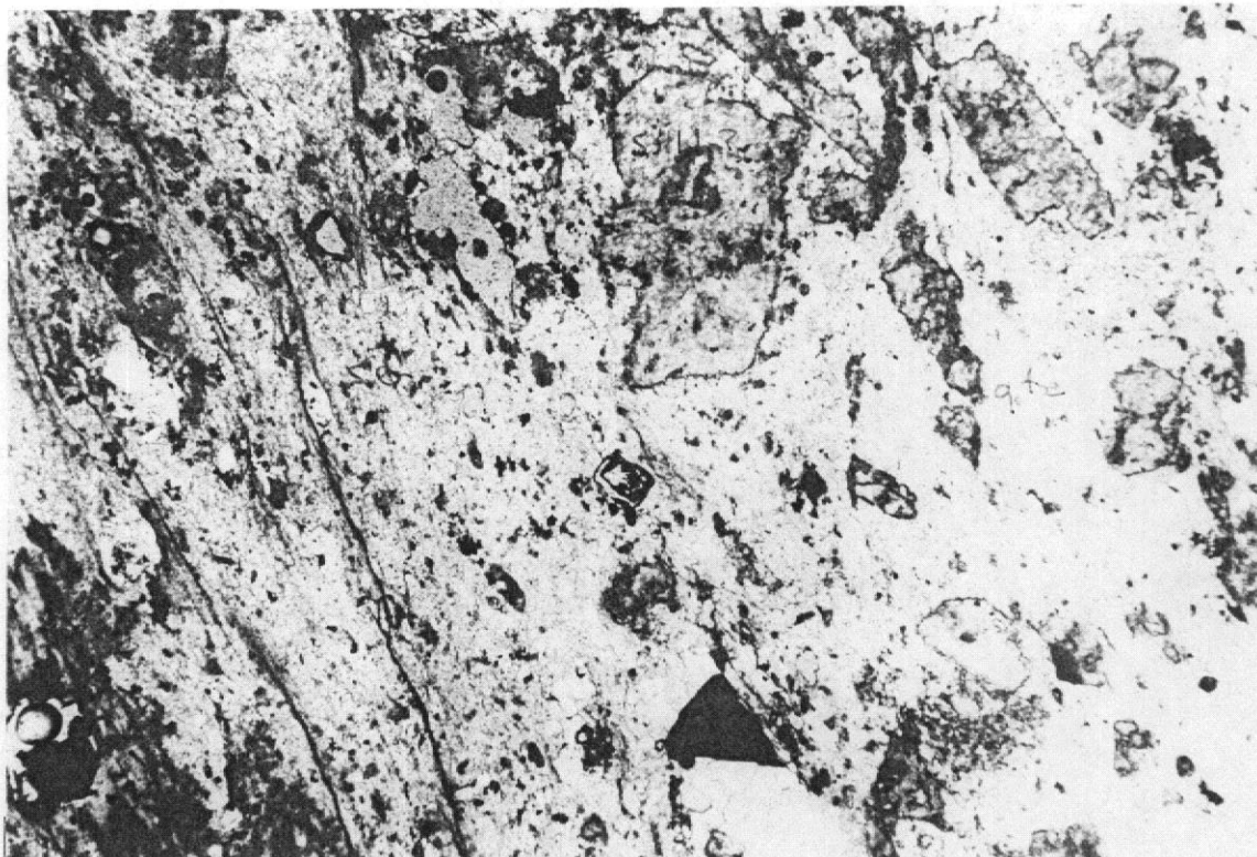
R99:12032. Fine grained foliated sericite and quartz contains equant to tabular sillimanite (?) after kyanite (?). Iron oxide after pyrite. Transmitted light, magnification 25x.
