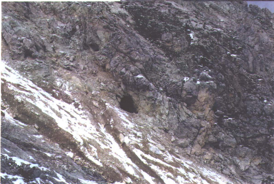
Photograph 26: Mountainview Adits: one of the more than 6 adits in the Mountainview area ~ 500m NE of Mt. Wirth, note eastward dipping limestone, higher angled shear through adit roof, immediate lower left corner of photo most likely shallow dipping fault surface
