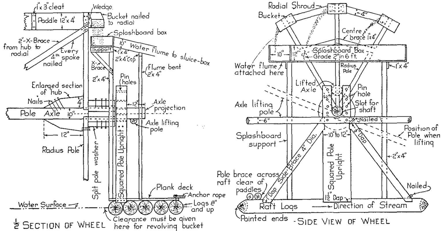
Fig. 5. Sections showing construction of parts of current wheel.
