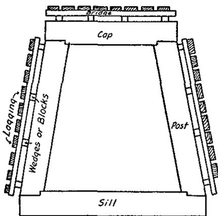
Fig. 6. A full set showing posts, cap, sill, wedges, bridges, and lagging. This is a breast set right up at the face of the working, with the lagging resting on the bridges. During the excavation of the next set-length the lagging is pushed through the spaces between the bridges and posts and cap and driven ahead.
