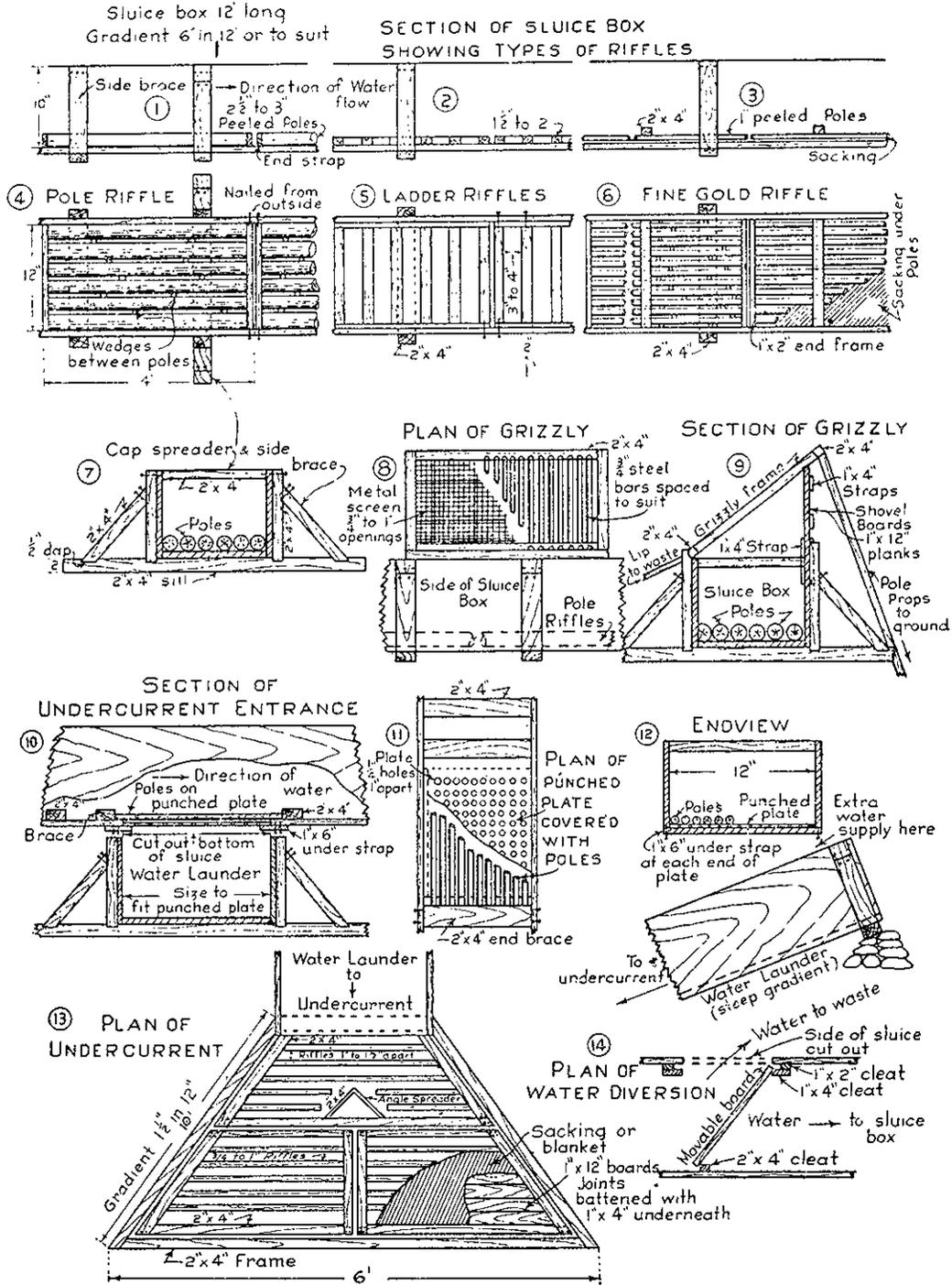
Fig. 4. Types of riffles, grizzly, undercurrent, and water diversion.
