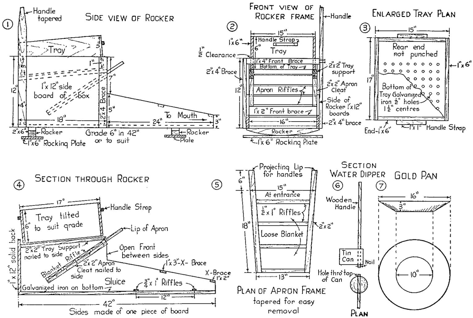
Fig. 3. Plan and sections of rocker, dipper, and gold-pan.
