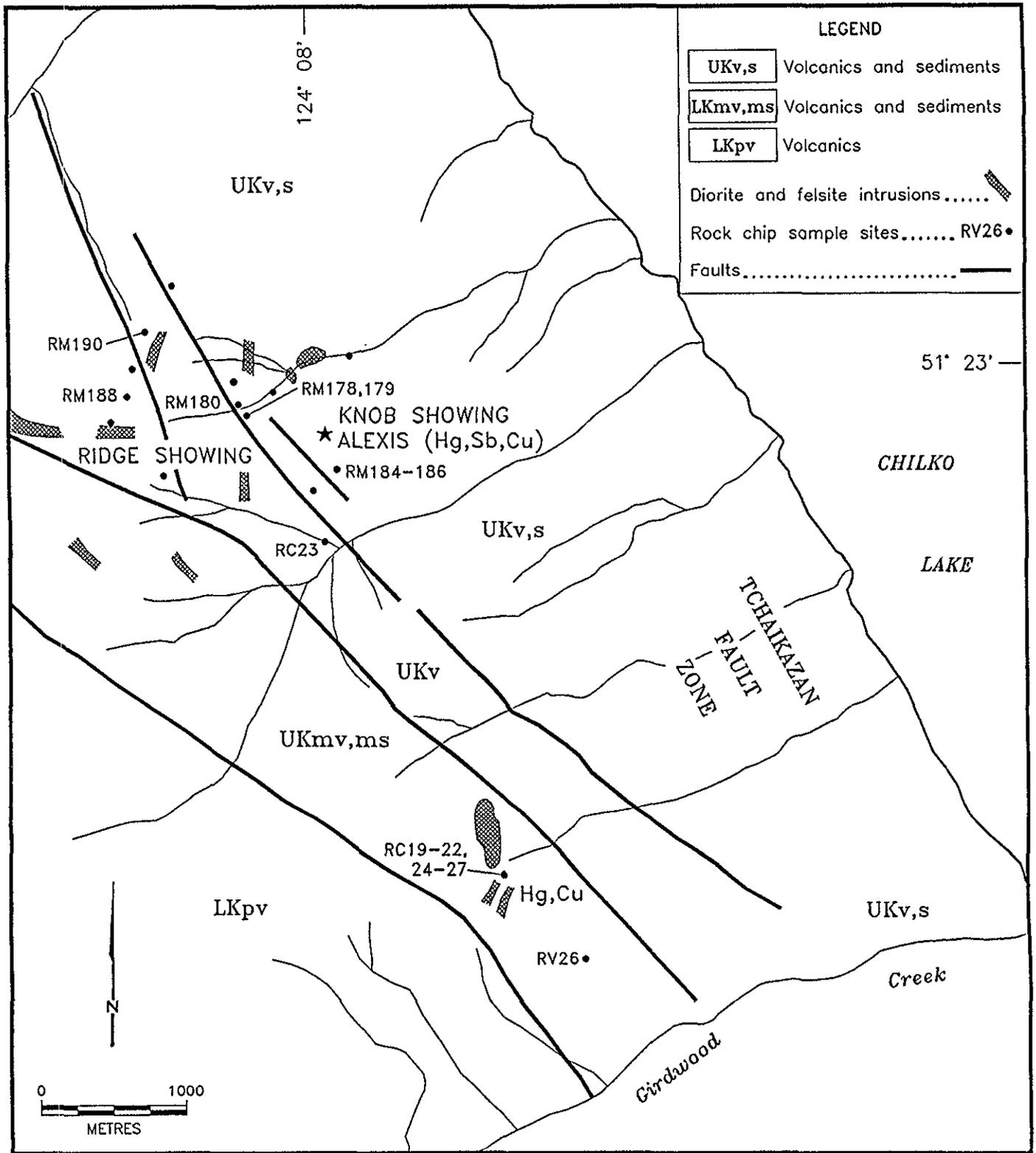
Figure 26. Geological setting of the Alexis mercury-copper showings.
