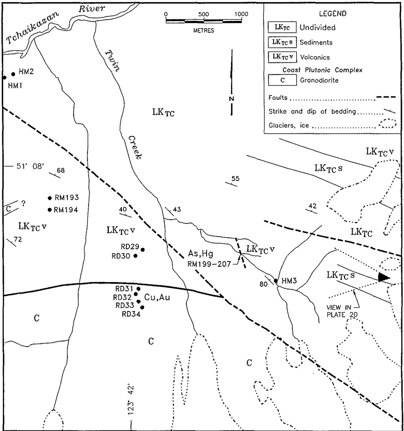
Figure 27. Geological setting of the Twin Creek area.
