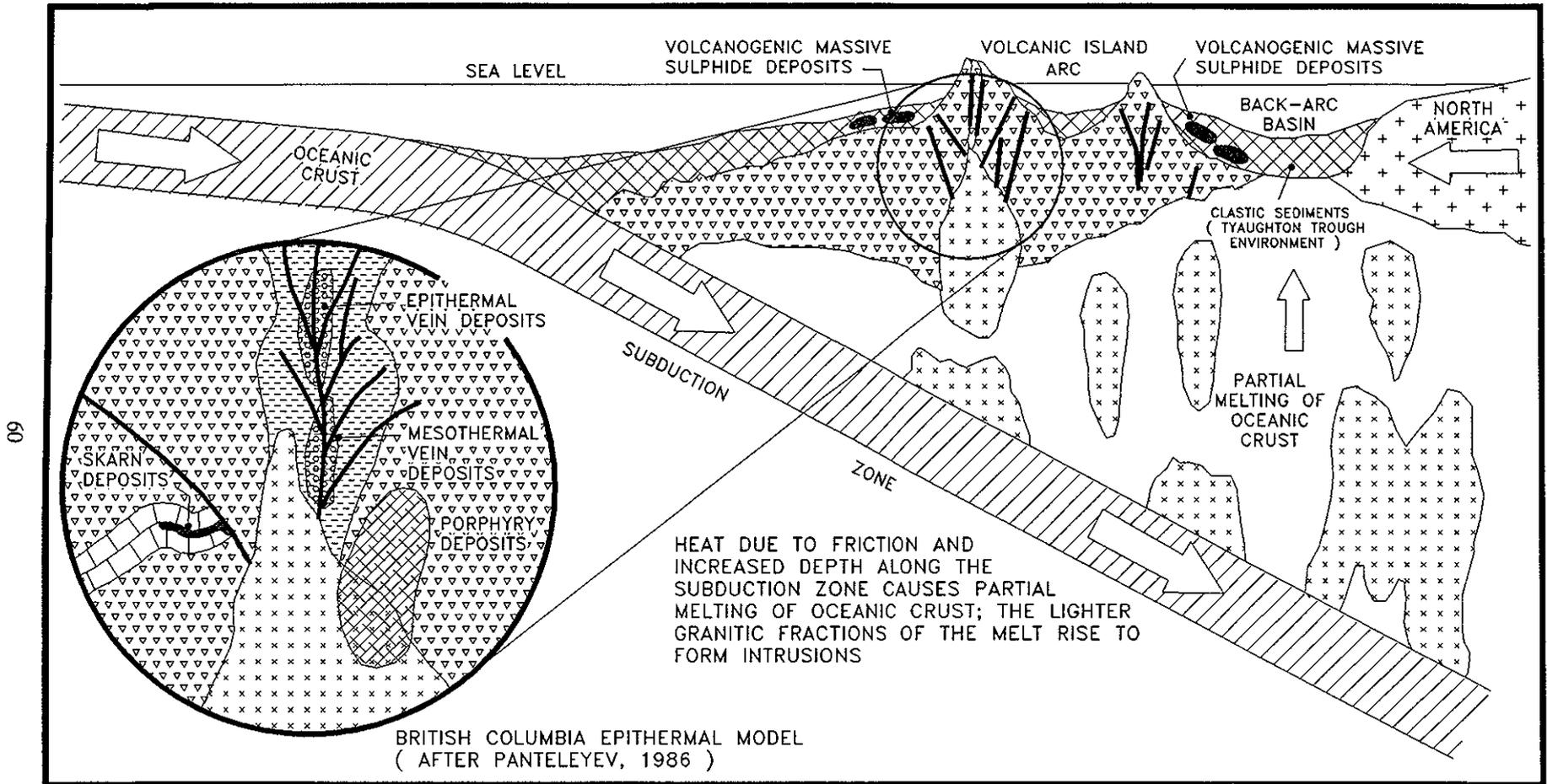
Figure 22. Conceptual models of mineral deposit genesis at convergent plate margins.
