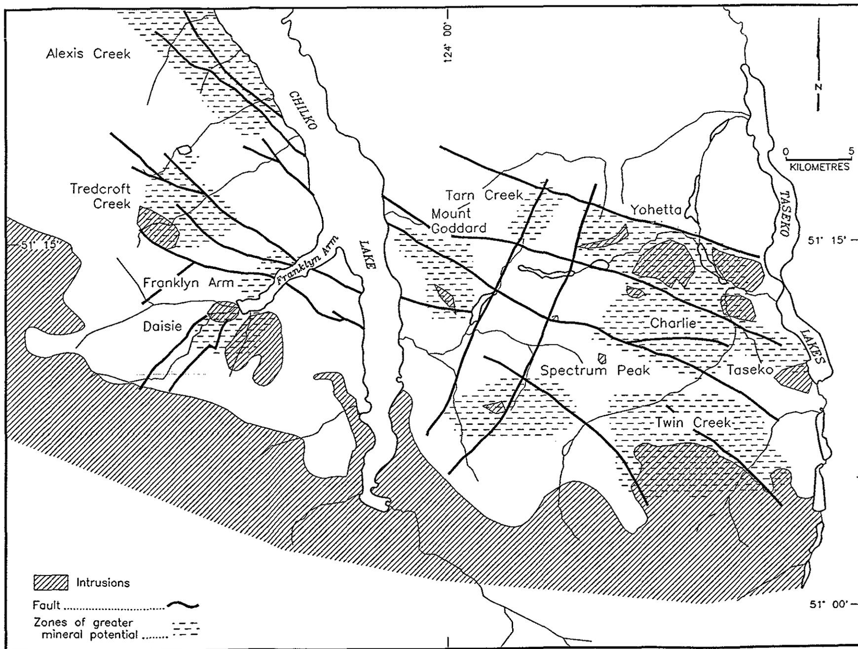
Figure 16. Zones of greater mineral potential as defined by stream-sediment geochemistry.
