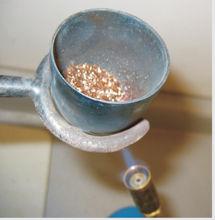
Figure 10. Crude laboratory set up used to exfoliate vermiculite-bearing rock samples taken from the outcrop adjacent to the Hodgie rare earth zone.
