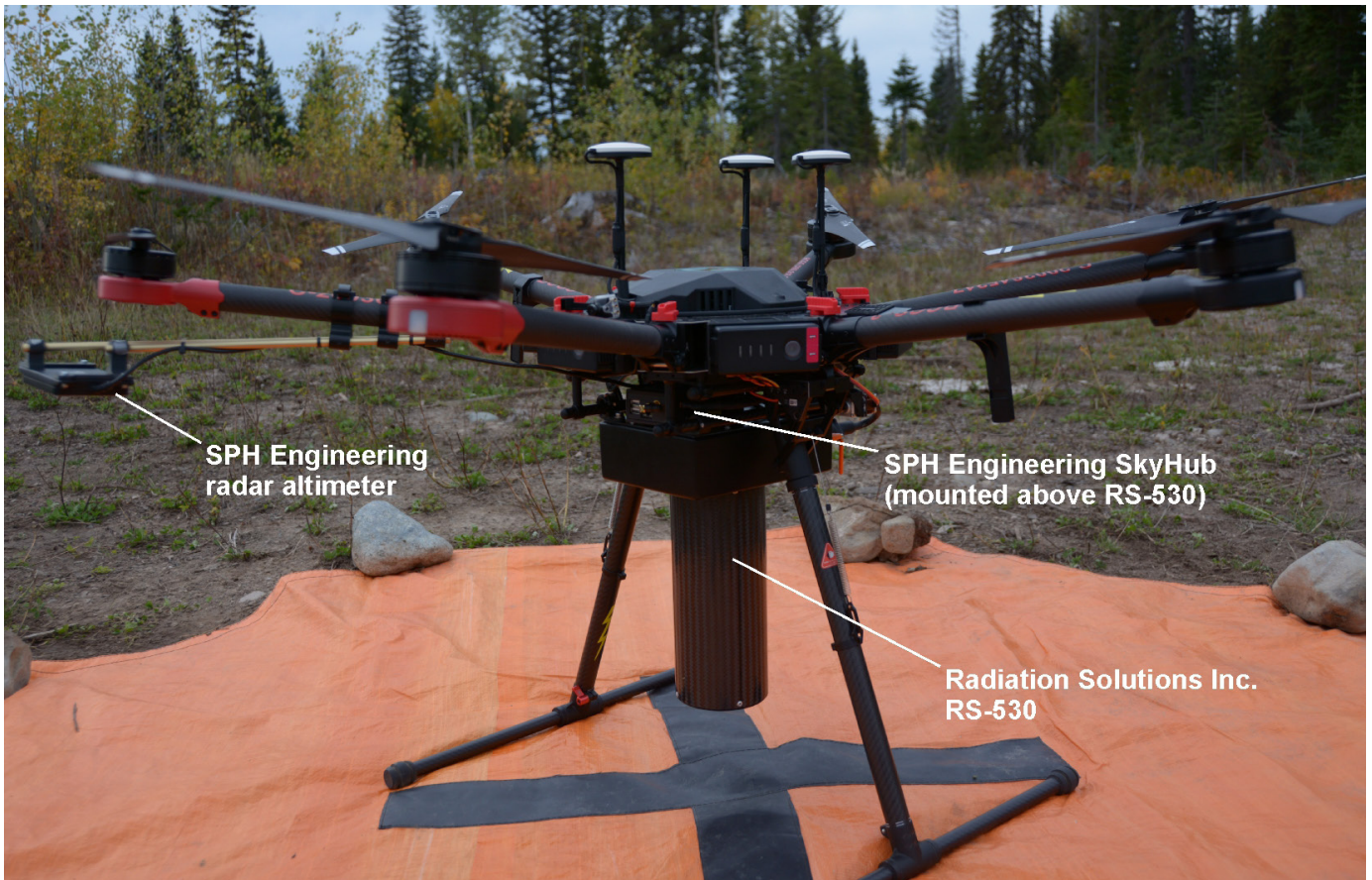
Fig. 7. DJI Matrice 600 Pro (M600) RPAS used to acquire lidar, magnetic, and radiometric data. A Radiations Solutions Inc. (RSI) RS-530 gamma-ray spectrometer is mounted beneath, above which is an SPH Engineering Skyhub onboard computer. An SPH Engineering radar altimeter (NRA24) is mounted on an arm.
