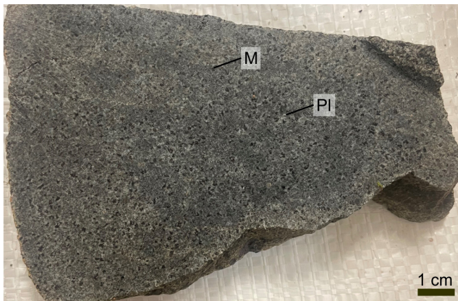
Fig. 13. Unassigned Late Cretaceous plutonic suite. Fine-grained biotite pyroxene diorite, sample RK23-117. M: mafic mineral, Pl: plagioclase
