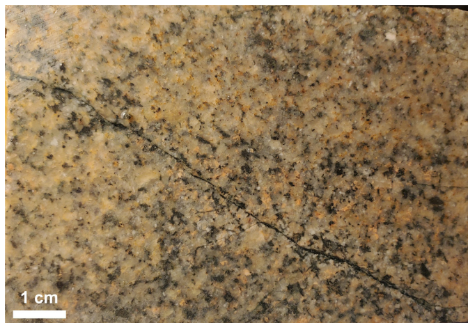
Fig. 4. Stikine plutonic suite, equigranular intrusions at the Schaft Creek deposit. Equigranular granodiorite from drill hole 08CF364 at 28.3-28.8 m (same lithology as sample 08CF364-31.7m).
