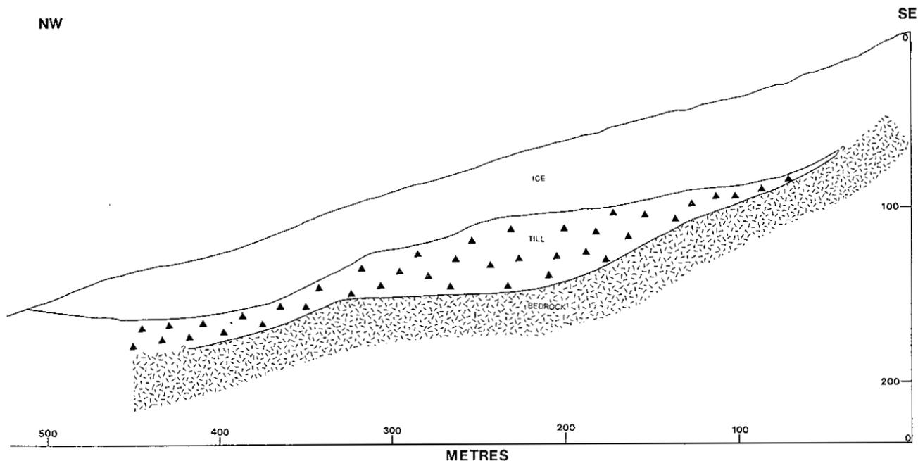
Figure B-7-9. Longitudinal section through Johnny glacier near its terminus, based on drill-hole data. Modified from Burlington *et al.*, (1985).
