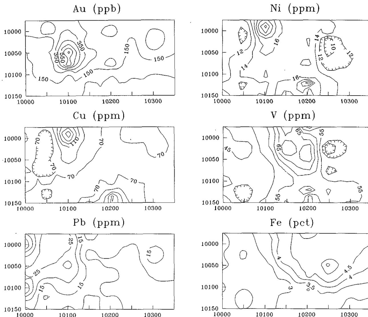
Figure B-4.3. Element dispersion patterns within the study area for Au, Cu, Pb, Fe, V and Ni. Down-slope direction in each diagram is from top to bottom.
