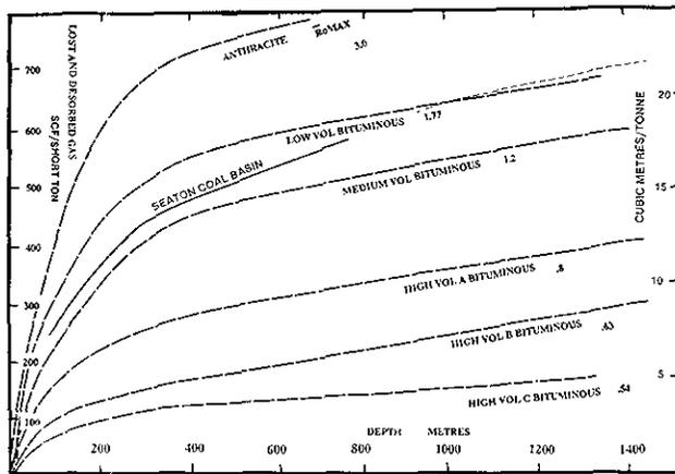
Figure B-8-8. Coalbed-methane retention track as a function of depth and rank for the Seaton coal basin.
