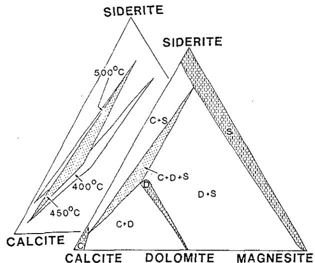
Figure B-1-1. Calcite-magnesite-siderite phase diagram. Valid for temperature of 450°C. D = dolomite, C = calcite, S = siderite - magnesite solid solution. Background diagram shows the position of the three-phase (C+D+S) triangles for temperatures of 400°C, 450°C and 500°C (after Rosenberg 1967).
