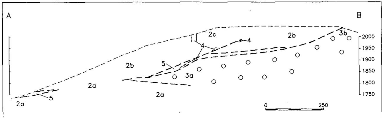
Figure B-2-2. Schematic cross-section showing relationship of the shear zone to geologic units. Legend as for Figure B-2-1.
