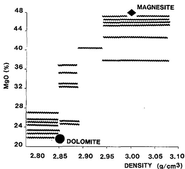
Figure B-1-3. The relationship between density and MgO content of carbonate rocks in the Mount Brussilof area.
