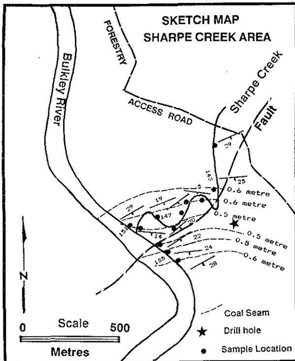
Figure B-8-4. Coal-seam distribution in the Sharpe Creek area.
