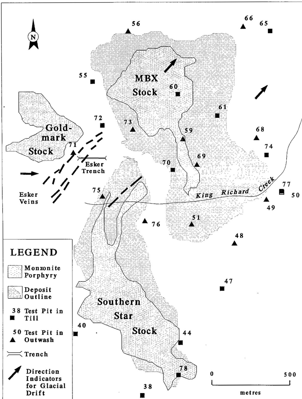
Figure B-6-3. Location of test pits and the Esker zone trench in relation to mineralization.
