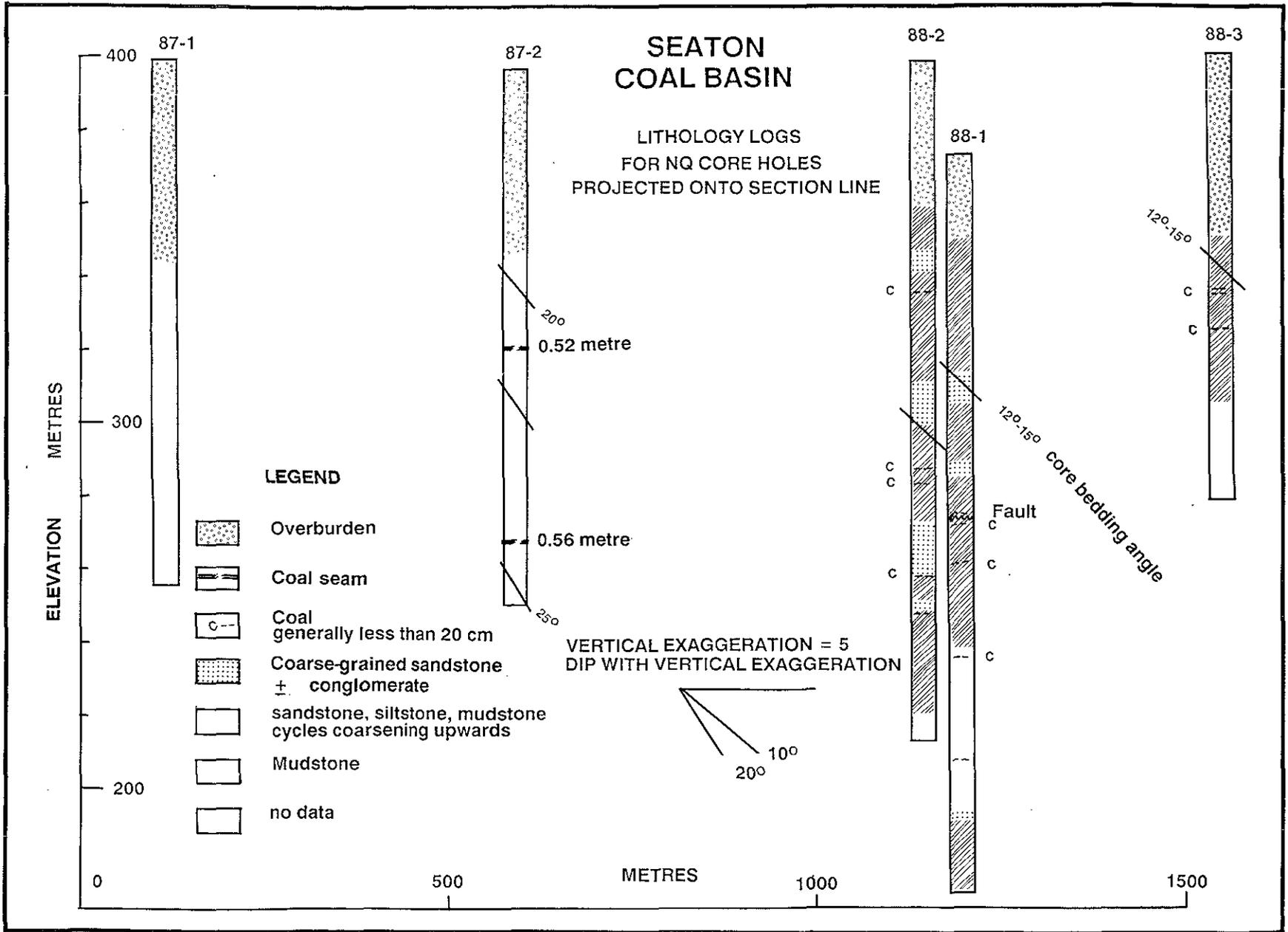
Figure B-8-5. Lithology logs projected onto section line A-B; Figure B-8-3.
