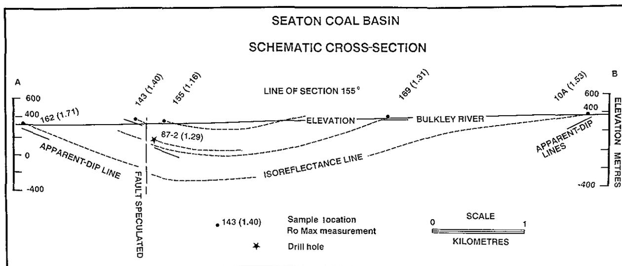
Figure B-8-7. Schematic cross-section of the Seaton coal basin showing reflectance data and apparent dip lines.
