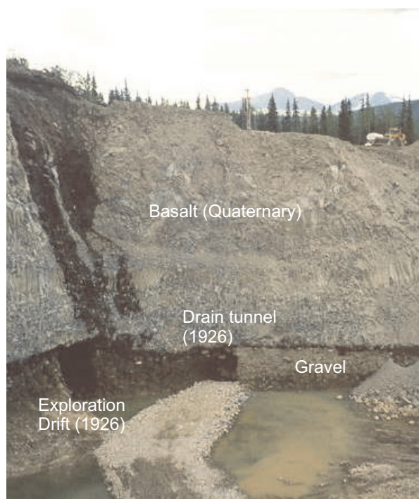
Photo 3. Rich paygravel in the old channel of Ruby Creek excavated beneath columnar-jointed basalt; two old underground drifts can be seen.
