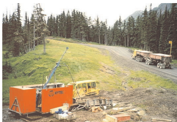
Photo 2. Exploration holes in the NEX zone are routinely drilled to 1500 metres. A truck departs the minesite carrying ore containing about $250 000 in gold and silver, destined for the DOWA or Noranda smelters.
