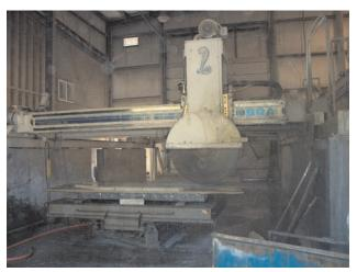
Photo 3. Gang saw cutting granite slabs at Garibaldi Granite Group Inc.'s dimension stone plant, Squamish.
