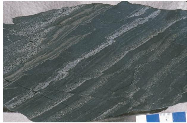
Photo 2. Eskay Creek ore, fine sulphosalt-sulphide beds in mudstone
