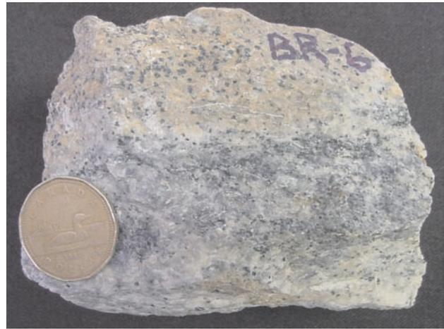
Photo 2. Aluminous alteration at the Briton iron prospect. The upper (beige-orange) layer consists of quartz, pyrophyllite, andalusite and minor nacrite. The lower (grey-blue) layer consists of corundum, quartz, pyrophyllite, andalusite and possibly nacrite.
