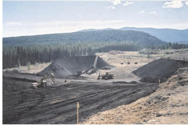
Photo 3. Basin Coal mine near Coalmont. The stripped but unmined coal seam is in the foreground with screened, raw coal on the pile near the conveyor. Photo courtesy of Eric Beresford, Compliance Energy Corp.
