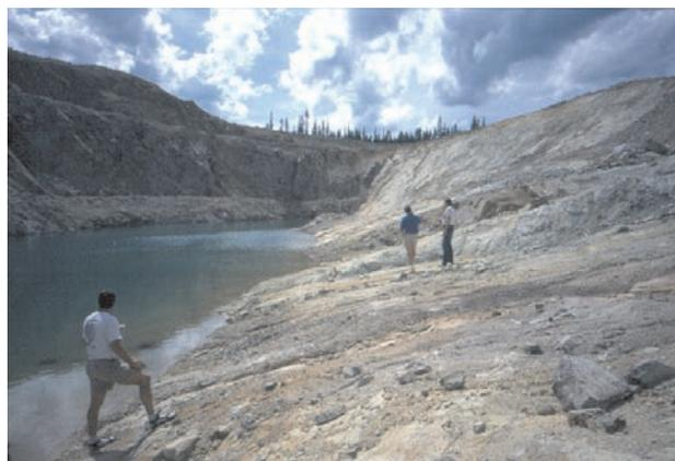
Photo 7. The Siwash North pit of Almaden Minerals Ltd. People are standing on the footwall of the mined-out vein.
