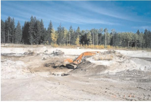
Photo 4. Flat-lying diatomaceous earth deposit, Red Lake quarry, Western Industrial Clay Products Ltd.
