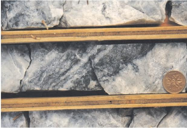
Photo 10. Close-up of core from Ted vein (hole TT-10) showing banded, fine-grained sulphides and sulphosalts.
