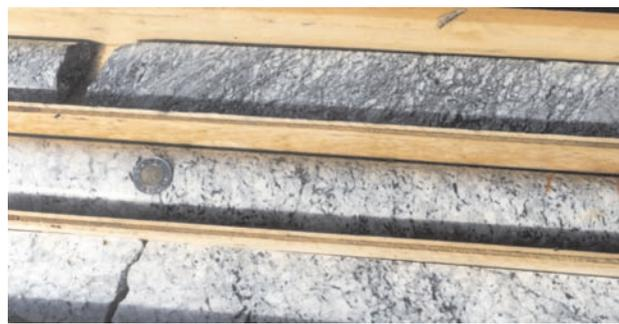
Photo 11. Tantalum, niobium and phosphate-bearing carbonatite in drill core from Commerce Resources' Fir property near Blue River (Hole 2002-7, 67m).
