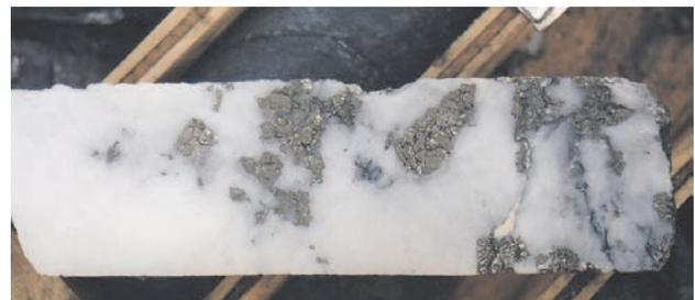
Photo 11. Quartz-pyrite vein mineralization from the Myrtle property.
