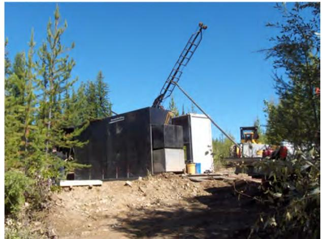
Figure 10. Diamond drilling on Astral Mining Corporation and Kootenay Gold Inc's Jumping Josephine property.
