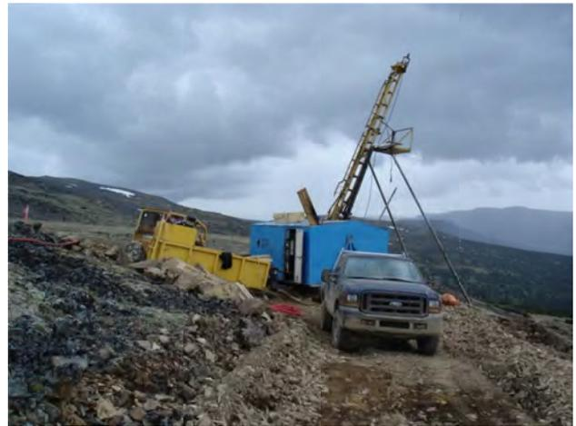
Figure 23. Diamond drill at Capoose in the Fawnie Range.
