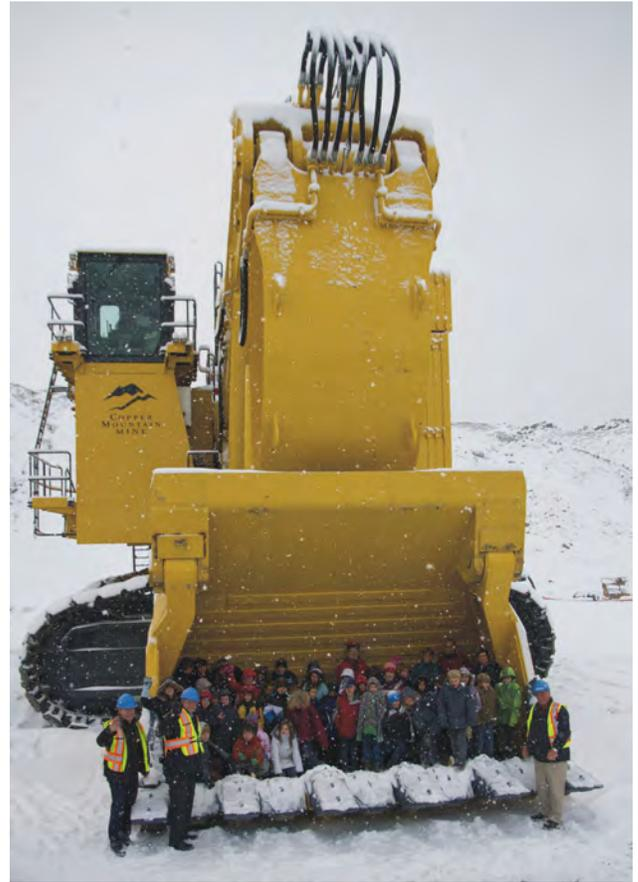
Figure 12. The first massive Komatsu PC 8000 production shovel was commissioned at the Copper Mountain mine development site in November, 2010 (photo courtesy of Copper Mountain Mining Corporation).
