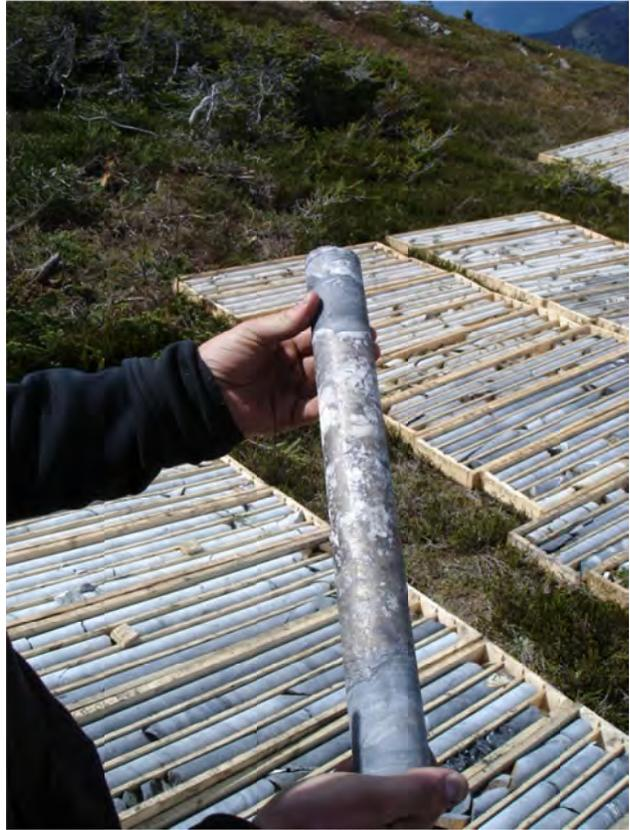
Figure 82. Maroon Mountain project; drill intercept of the auriferous Bear quartz-galena-sphalerite vein.
