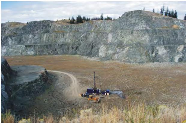
Figure 15. Abacus Mining and Exploration Corp and partner KGHM Polska Miedz S.A. are advancing the Ajax copper-gold project near Kamloops through to a feasibility study. Photo of drilling in the previously mined Ajax East pit which will be incorporated into a larger pit (file photo).
