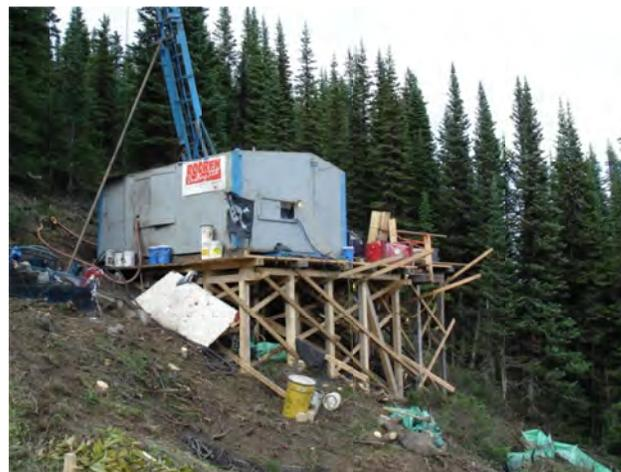
Figure 27. Akie, large drill platform to support a drill rig for deep holes.
