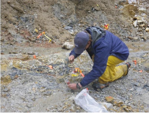
Figure 6. Channel sampling at Brocade Metals' Ruby Project (courtesy Brocade Metals).
