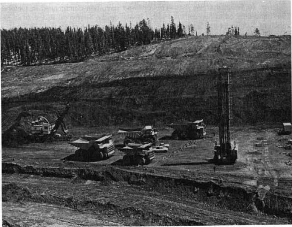
Plate XIa.—Kaiser Resources Ltd.'s Harmer No. 1 open pit with several 200-ton capacity Lectra Haul dump trucks. (Courtesy Kaiser Resources Ltd.)
