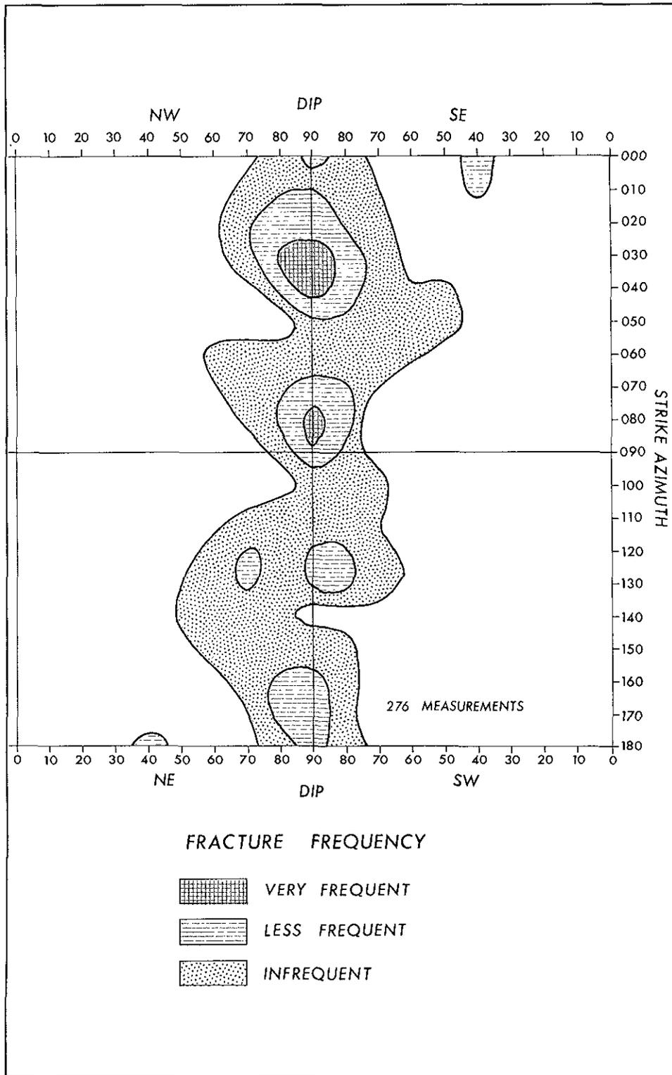
Figure G-44. Fracture frequency plot for the Hat Creek area. G 113
