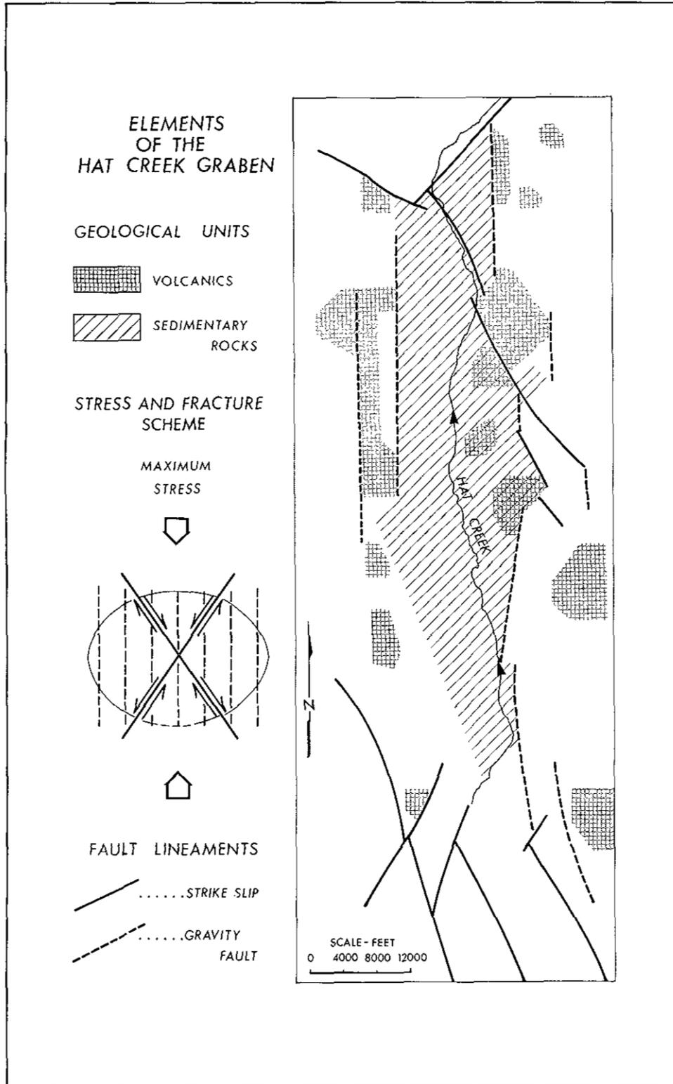
G 112 Figure G-43. Possible stress scheme relating faulting to graben development in the Hat Creek area.
