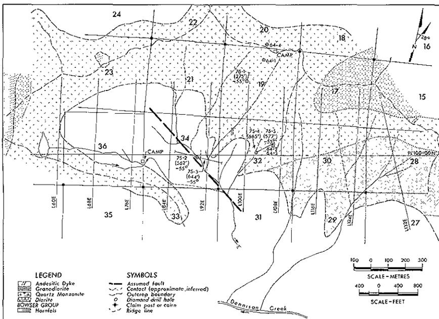
Figure G-33. Geology of the Den copper prospect (after company plans).
