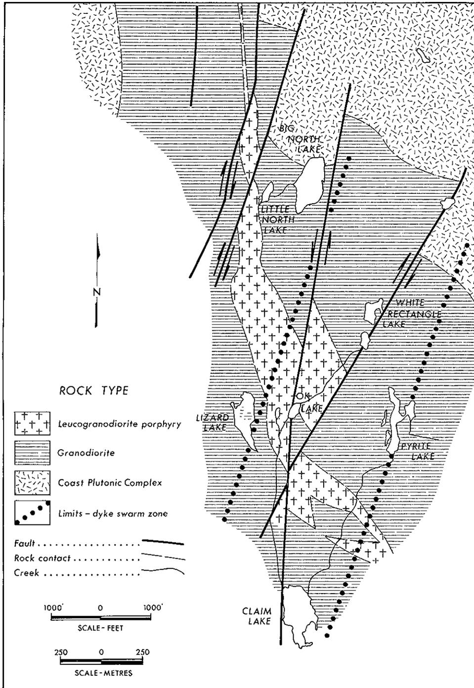
Figure G-25. Geology of the OK deposit (from Meyer, Gale, and Randall).
