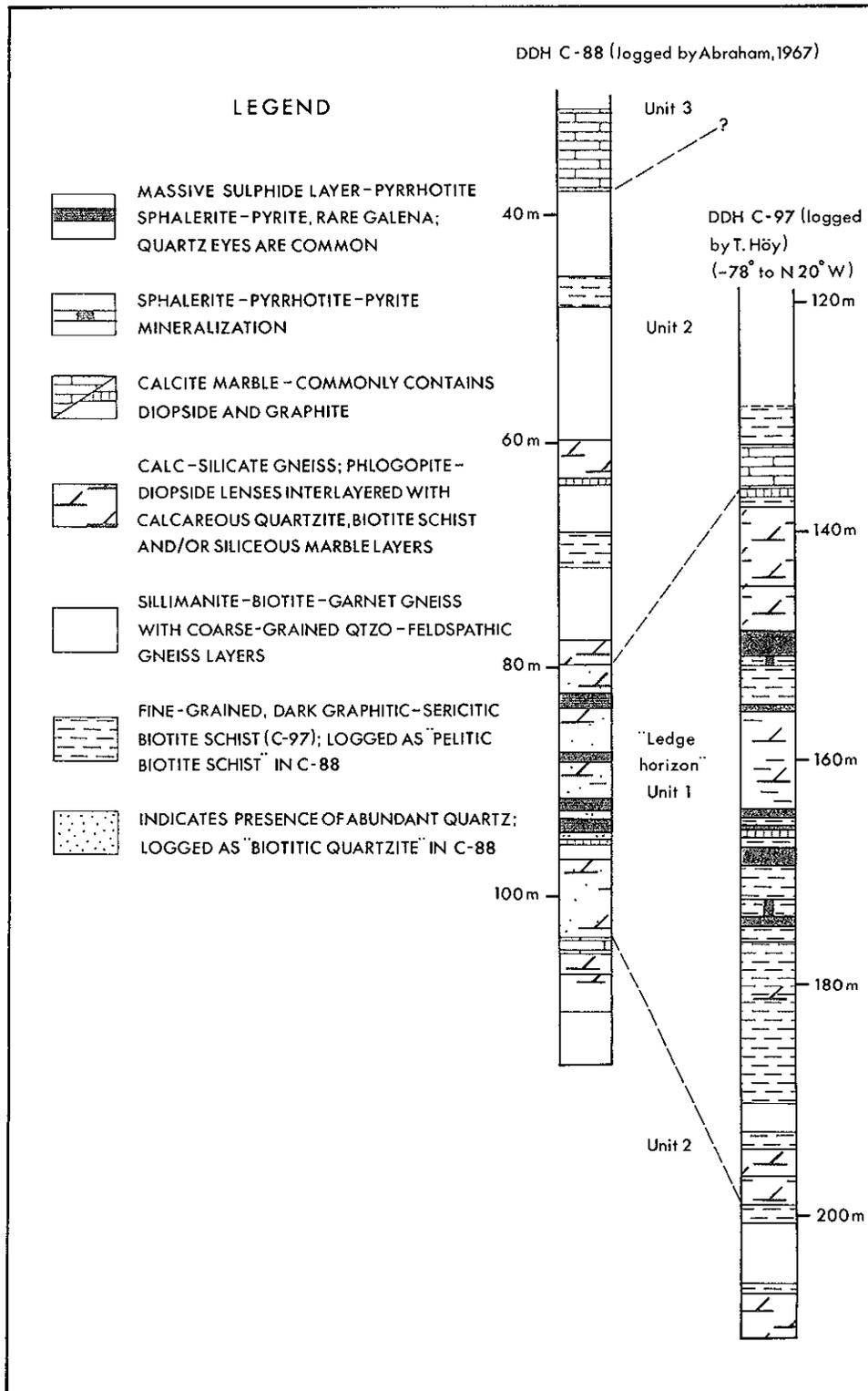
Figure G-10. Drill hole sections through the Big Ledge.
