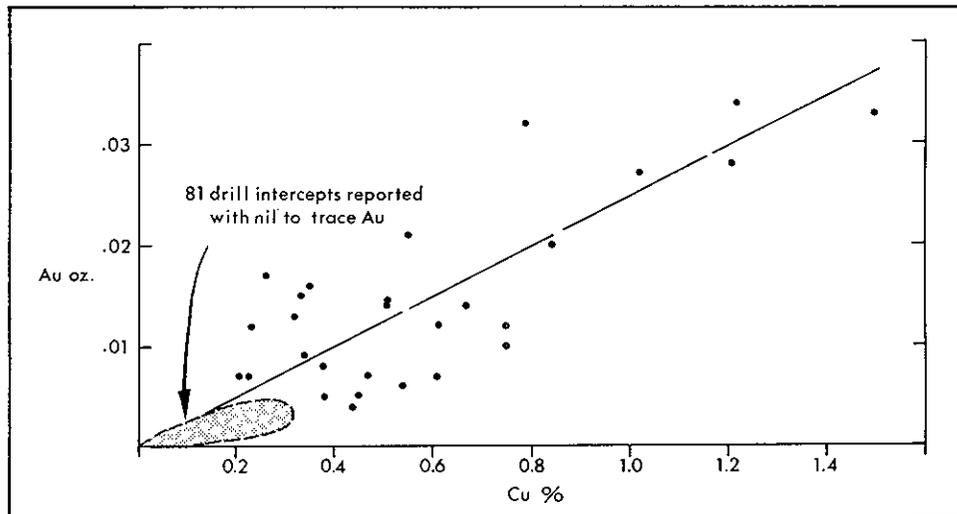
Figure G-37. Relationship of gold and copper in diamond-drill cores (Chris, Red, Sus, Windy) (plot of 109 drill intercepts from 49 core and 24 percussion-drill holes).
