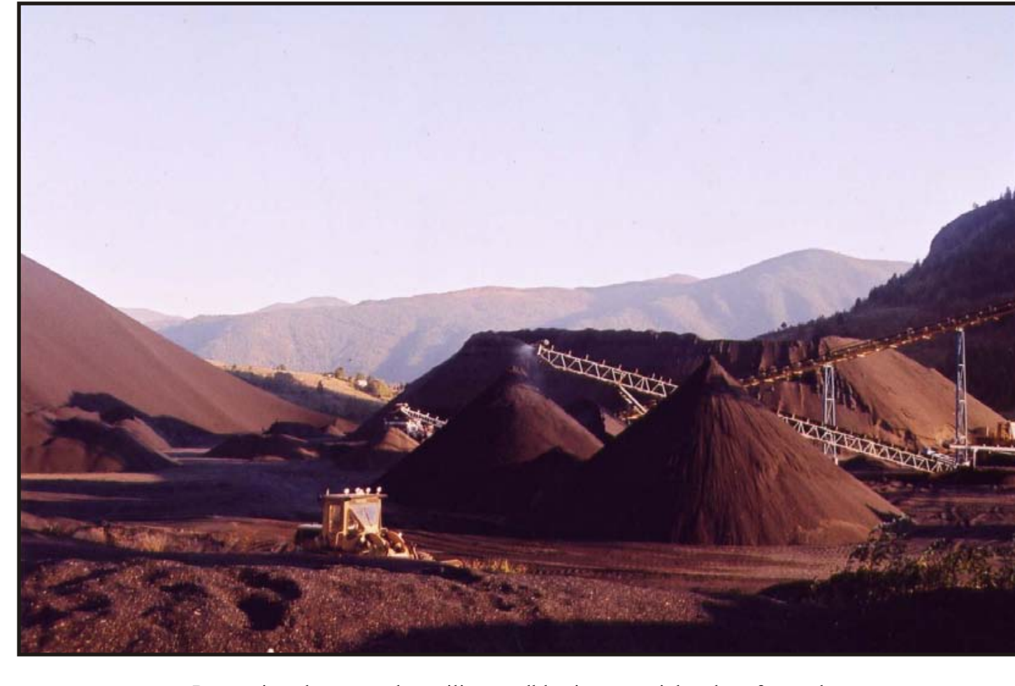
Processing slag to produce silica sandblasting material and roof granules, Pacific Abrasives & Supply Inc. mill, just north of Grand Forks.
