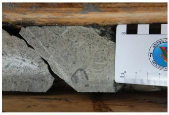
**Fig. 2.** Silicified (±sericitized) Nicola Group crystal-lithic tuff with disseminated pyrite. This type of rock has returned significant gold values in Lightning zone intersections. Tower Resources Ltd., Rabbit North project.
