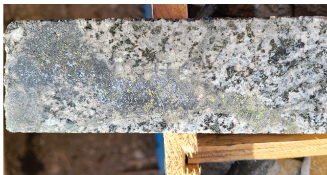
Fig. 7. Drill core showing chalcopyrite, pyrite, and molybdenum in veinlets within a porphyry unit, Bergette target. Photo courtesy of Surge Copper.
