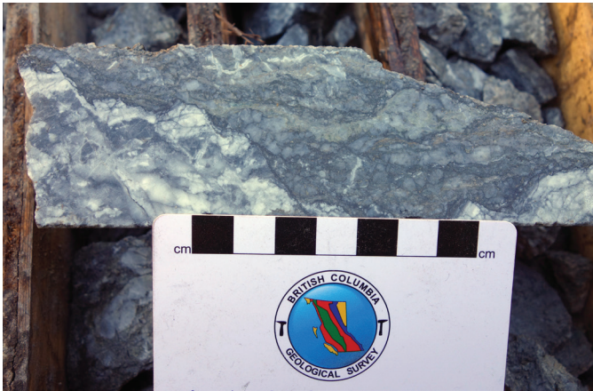
Fig. 3. Brecciated quartz veins and sulphides from a drill sample grading 16 g/t Au. Eagle zone, Reliance project, Endurance Gold Corporation.
