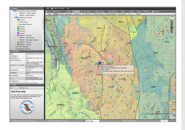
The MapPlace Map Window is bounded by several components. At the top is the Toolbar, which contains tools to navigate the map, zoom, create buffers, add points, lines, and polygons, query data, and select features. At the bottom is an Information Bar, showing scale, cursor location, and selection. On the left are three panes: Legend with selectable layers, Selection displaying data, and Tasks to access custom applications.
