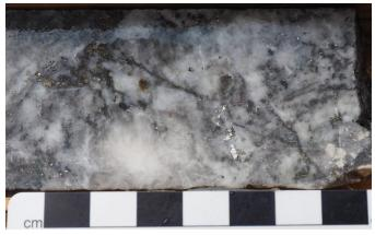
**Fig. 7.** Visible silver in core of a quartz-carbonate vein, Dolly Varden deposit. Kitsault Valley project (Dolly Varden Silver Corporation).
