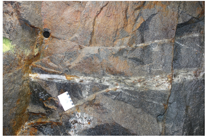
Fig. 5. Gold-bearing quartz-pyrrhotite veins in quartz diorite at Harrison Gold (Bear Mountain Gold Mines Ltd.).
