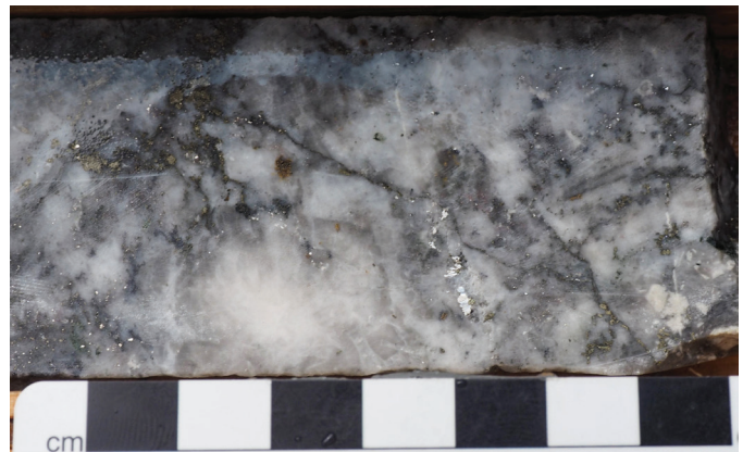
Fig. 7. Visible silver in core of a quartz-carbonate vein, Dolly Varden deposit. Kitsault Valley project (Dolly Varden Silver Corporation).
