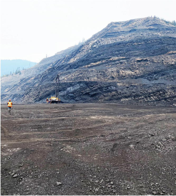
Fig. 4. Gently dipping coal-bearing Gething Formation strata, Willow Creek mine (Conuma Resources Ltd.).
