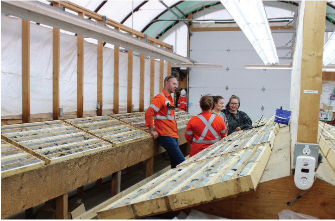
Fig. 2. Logging K-zone core at New Afton mine (New Gold Inc.).
