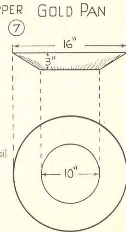
Plan and Sections of Rocker, Dipper, and Gold-pan.
