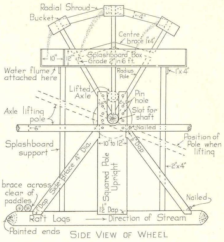
Sections showing Construction of Parts of Undercurrent-wheel.
