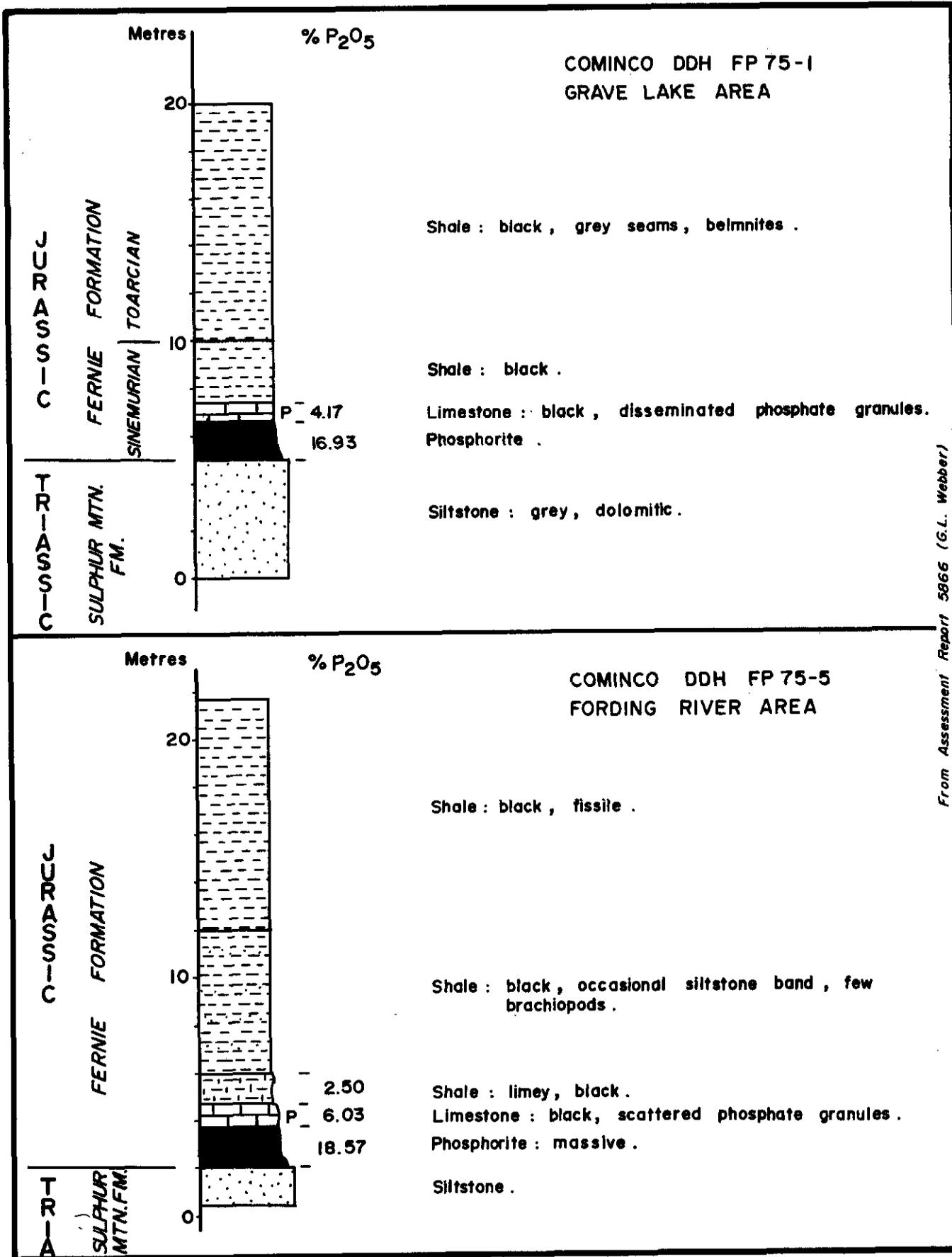
Figure 31. Diamond-drill hole sections, Fording River - Grave Lake area.
