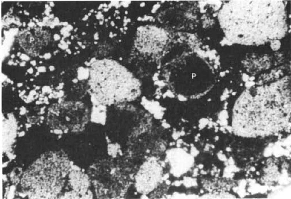
Plate 14. Photomicrograph (40x) of pelletal phosphorite, Mount Lyne. Phosphate pellets (P) with a compact texture occur in a quartz matrix.
