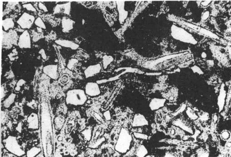
Plate 9. Photomicrograph (40x) of phosphate intraclast containing phosphate pellets (black), quartz grains (white) and shell material from Permian Ishbel Group, Crowsnest Pass area.
