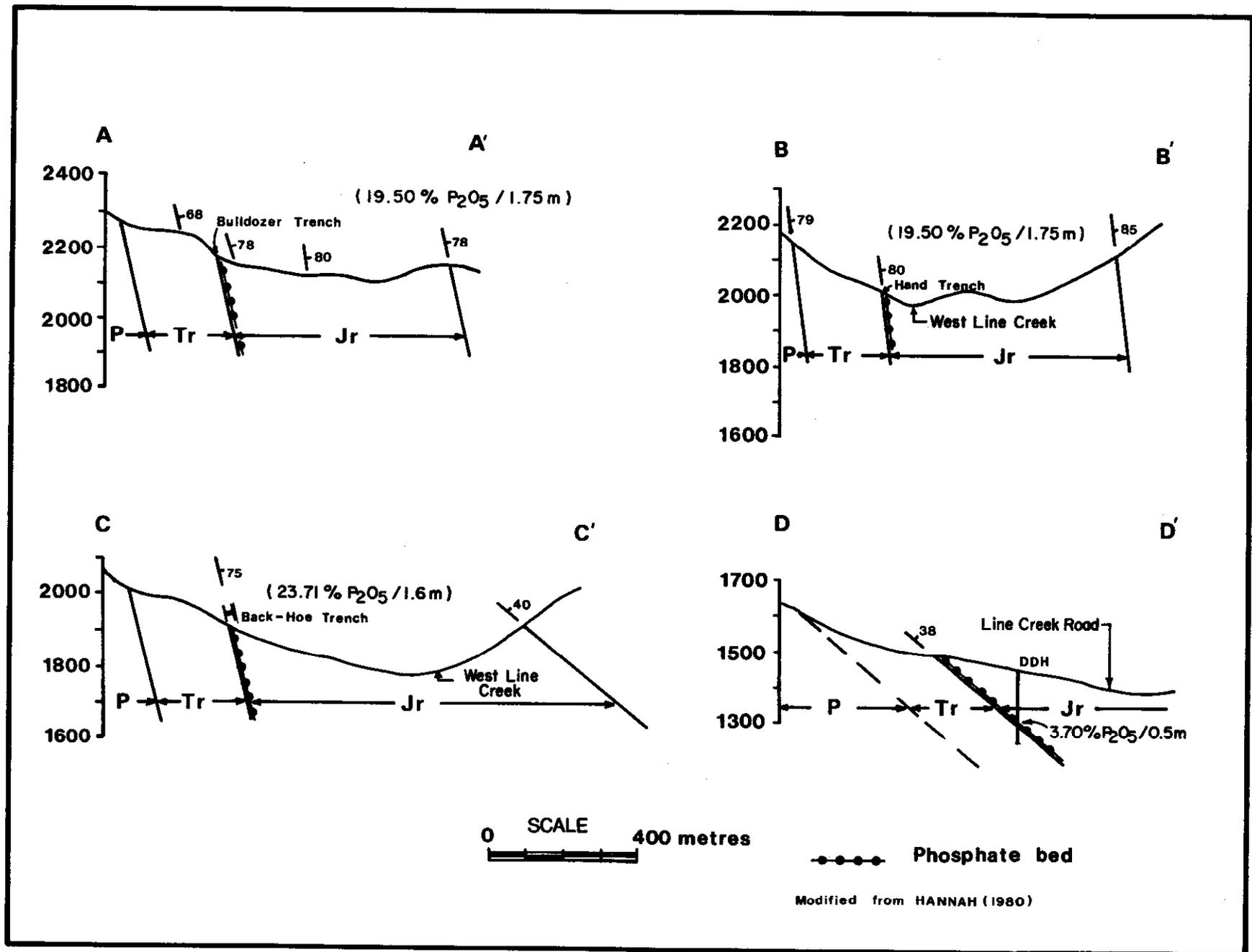
Figure 24. Cross-sections through basal Fernie phosphate, west Line Creek.
