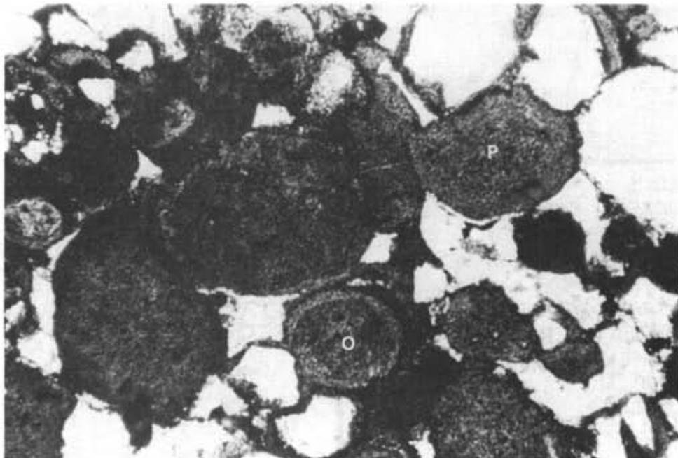
Plate 21. Photomicrograph (40x) of pelletal phosphorite, Fording River. Structureless pellets (P) and rare oolite (O) occur in a matrix of calcite and quartz.
