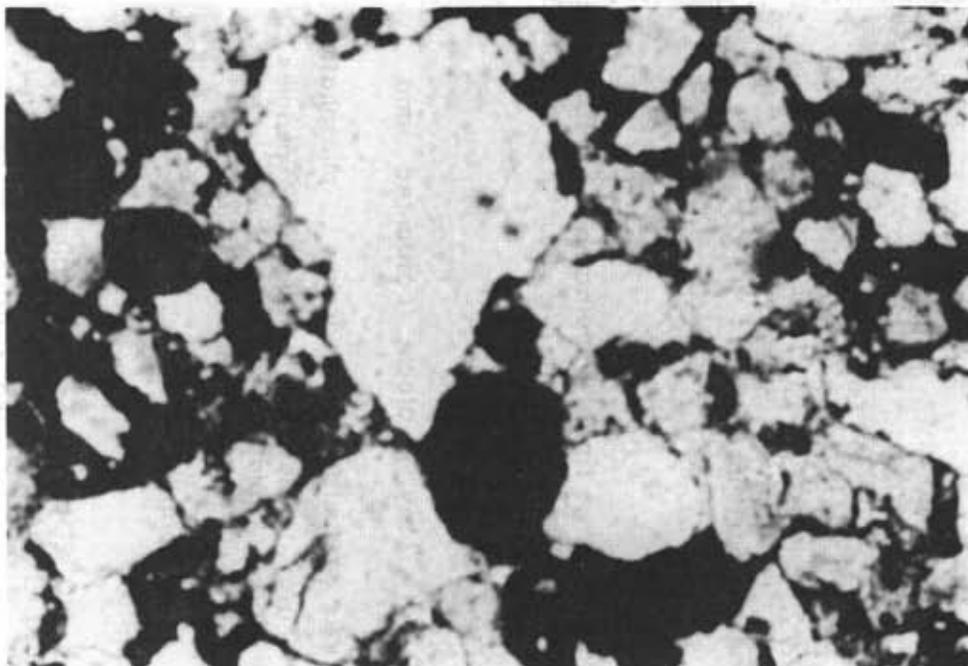
Plate 18. Photomicrograph (40x) of phosphate pellets (black) in a quartz (white) sandstone, Abby Ridge.
