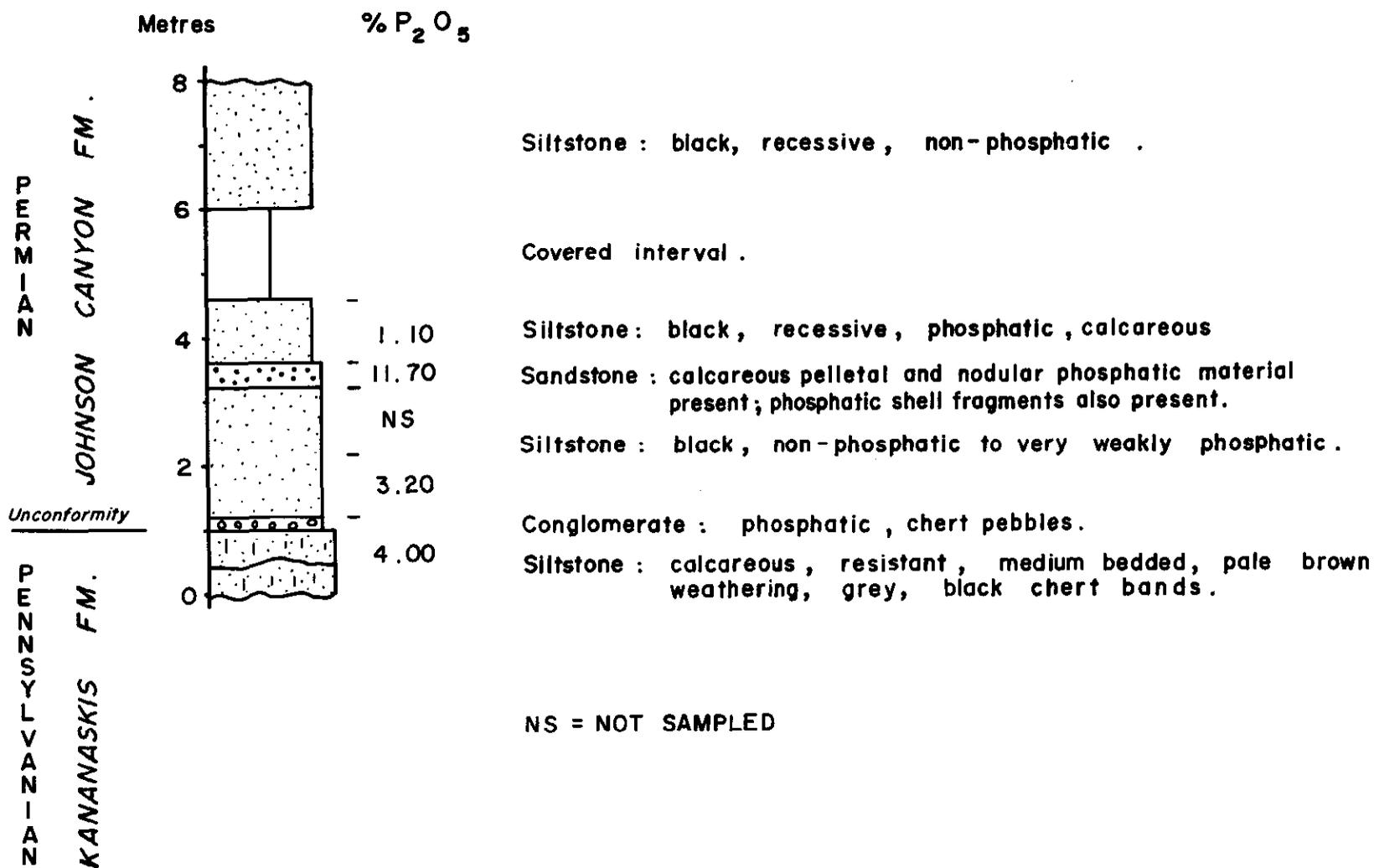
Figure 20. Stratigraphic section B4, MacDonald thrust fault at Fenster Creek.
