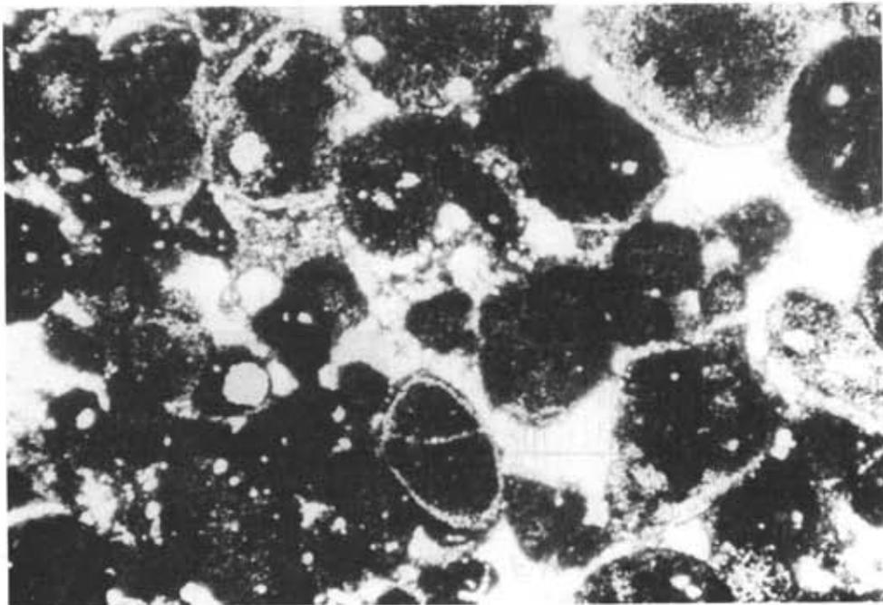
Plate 15. Photomicrograph (40x) of pelletal phosphorite from the Crow deposit. Pellets of fluorapatite occur in a matrix of quartz with minor calcite and lesser feldspar, illite and albite.
