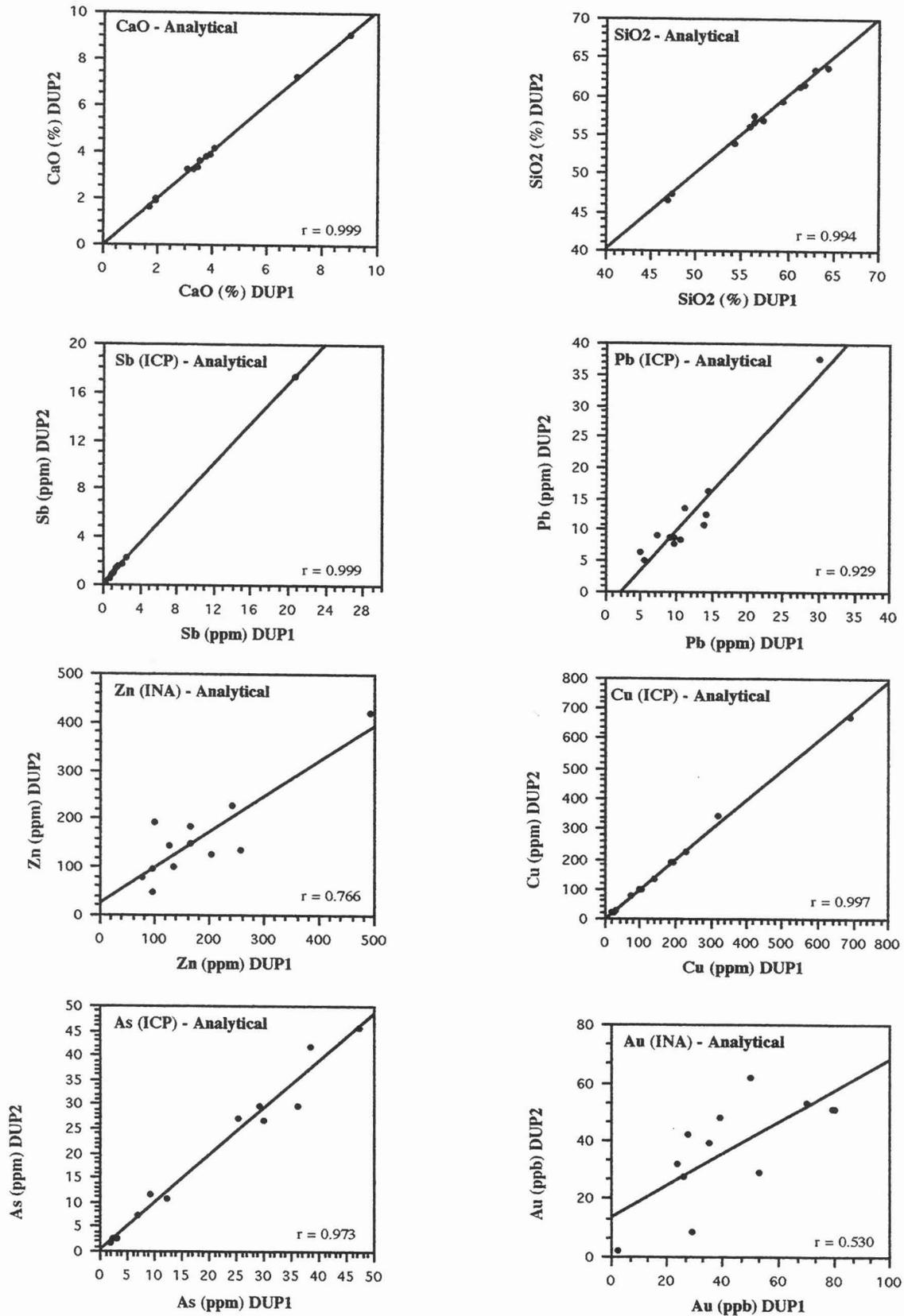
Figure 8. Bivariate scatter plots of analytical duplicate pairs for the Chu Chua - Clearwater till geochemistry study.
