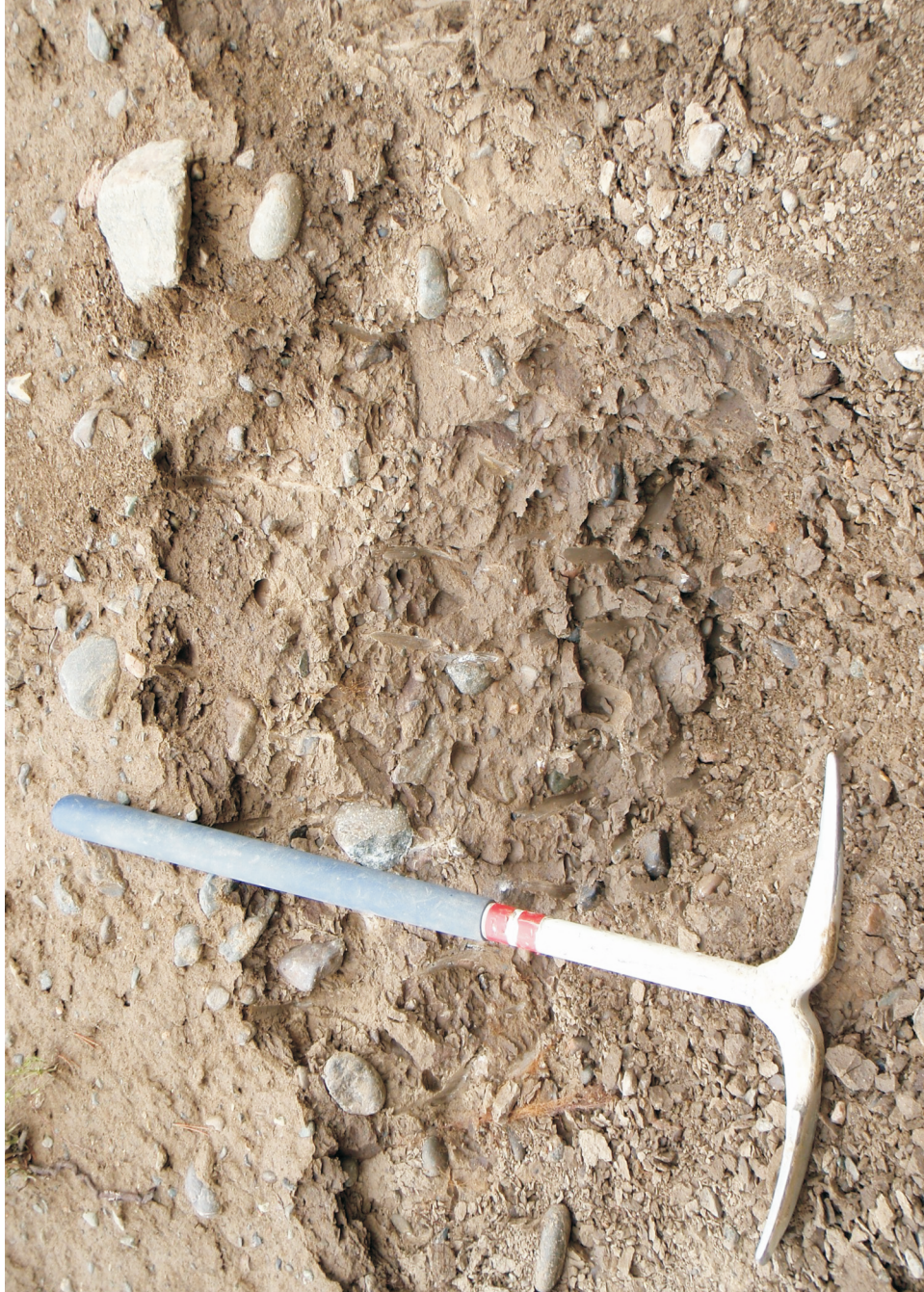
Figure 4. Silt and clay-rich, overconsolidated diamicton, interpreted as a basal till. Moderately well developed vertical jointing and subhorizontal fissility give this basal till a blocky appearance. Pick for scale (65 cm).
