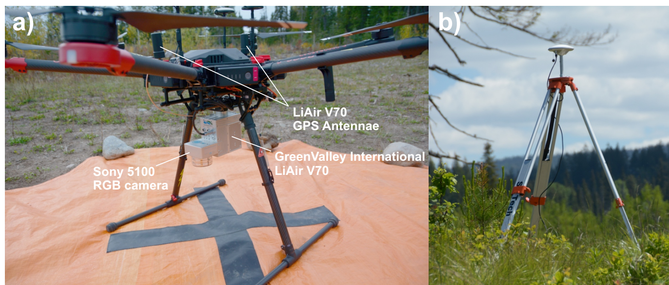
Fig. 2. RPAS platform and lidar scanner. a) Green Valley LiAir V70 (including RGB camera module) mounted on a DJI Matrice 600 Pro aircraft. The two LiAir V70 external global navigation satellite system antennae are mounted to the top of the aircraft. b) LiAir V70 global navigation satellite system base station.
