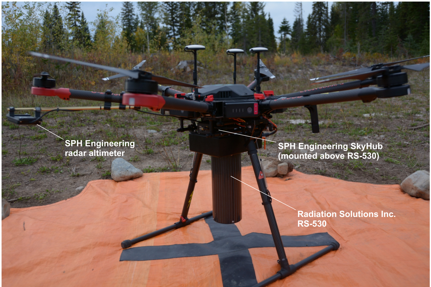
Fig. 8. DJI Matrice 600 Pro (M600) RPAS. The RSI RS-530 gamma-ray spectrometer is mounted to underside of M600. An SPH Engineering radar altimeter is mounted to a forward motor boom and communicates through the Skyhub to flight controls to maintain a constant altitude above ground during autopilot surveys.
