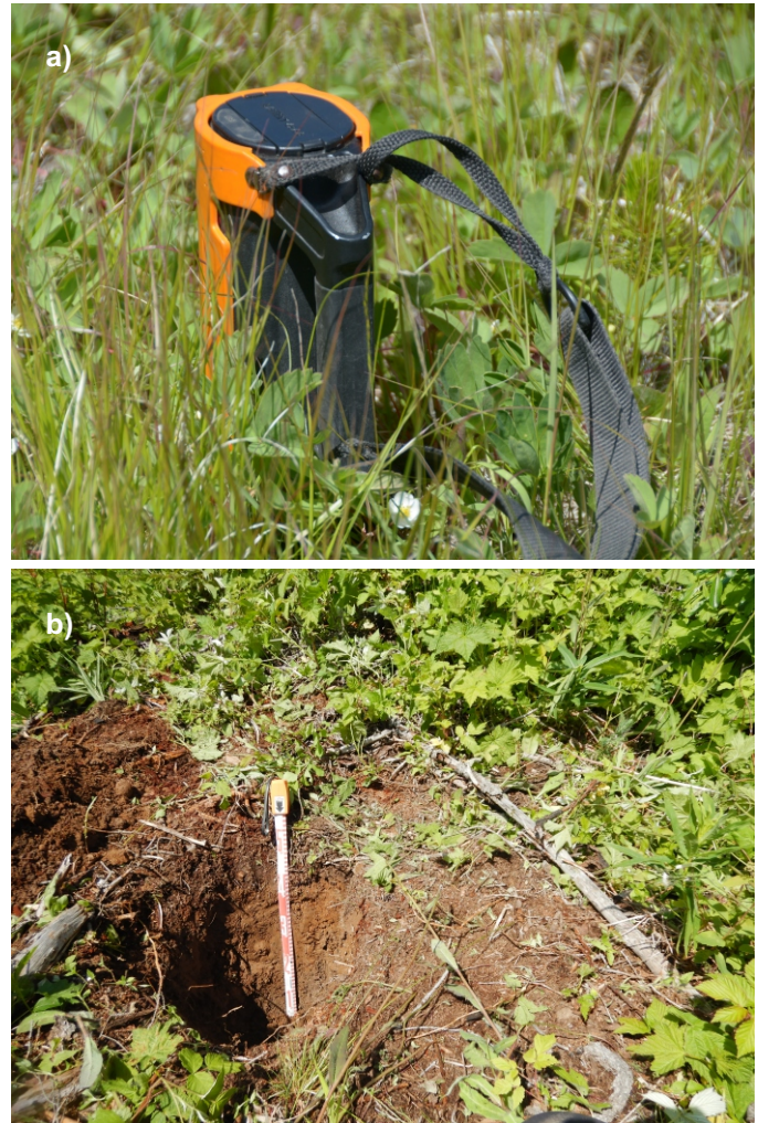
Fig. 9. a) RSI RS-230 BGO Super-SPEC (RS-230) handheld gamma-ray spectrometer used to collect ground radiometric data. b) Typical 50 cm deep soil pit dug to observe the soil profile measured by the RS-230.
