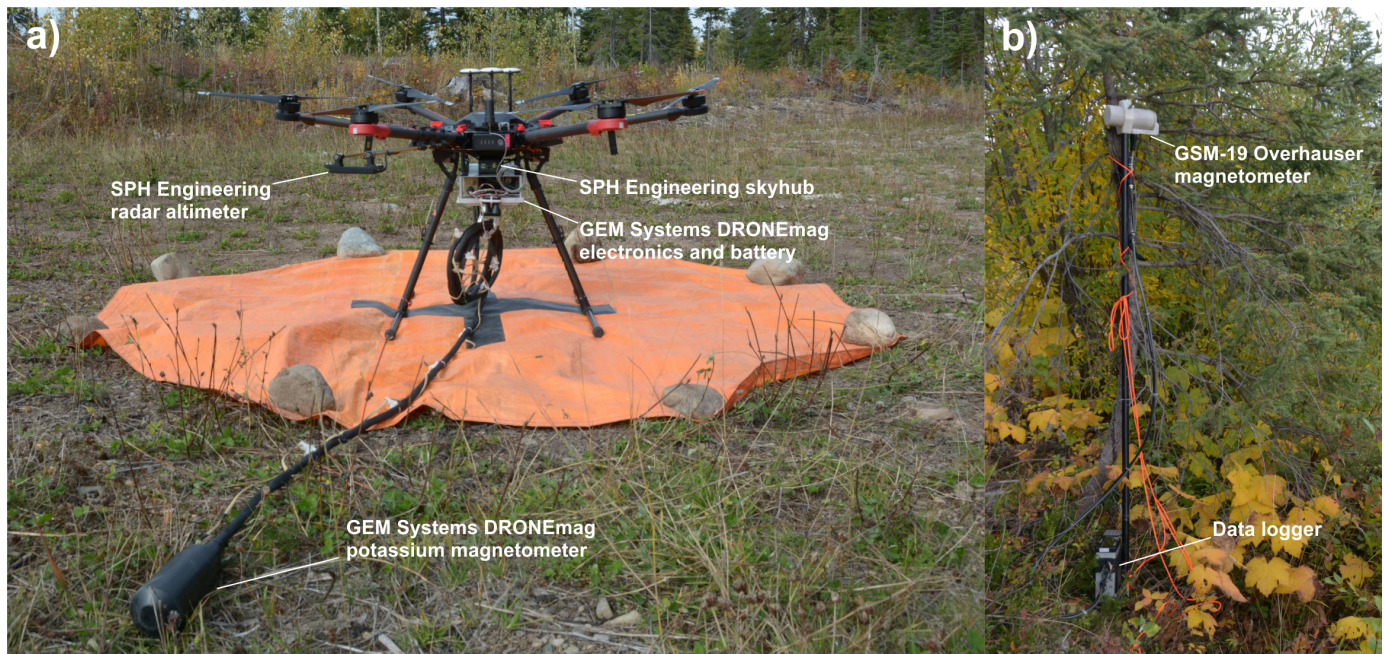
Fig. 4. RPAS magnetometer acquisition equipment. a) GEM Systems GSMP-35 U (DRONEmag) potassium magnetometer mounted on a DJI Matrice 600 Pro. The instrument's electronics and battery are housed in a custom tray mount. The magnetometer sensor is slung 2.5 m from the mount's base. b) GSM-19 Overhauser magnetometer attached to a tree; data logger at base.
